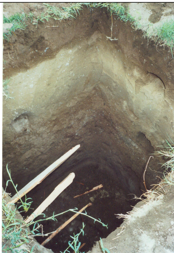
j) Soil pit showing the moisture profile
