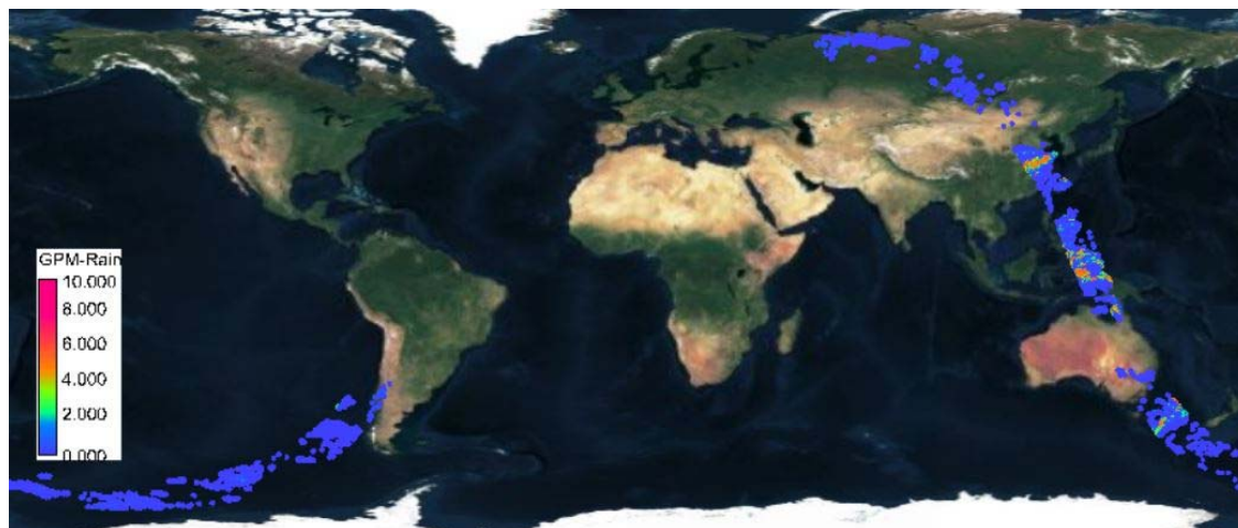
Figure 3.14: GPM derived precipitation in orbit configuration for 1 hr duration
