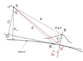
Point **B** with elevation **h** above the ellipsoid is imaged at position **B'** in SAR image, though its real position is **B''**. The offset  $\Delta r$  between **B'** and **B''** exhibits the effect of topographic distortions
