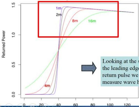
Looking at the slope of the leading edge of the return pulse we can measure wave height!
