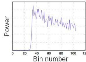
SAR wave-form much more « peaky » than Brown's wave-form (because of surface reduction from internal to external rings)
