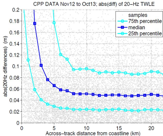
Figure 6: scatterplot of the absolute value difference between consecutive TWLE measurements against **across-track** distance from coast, and the statistics of its distribution in 1-km distance bins, for the CPP dataset.
