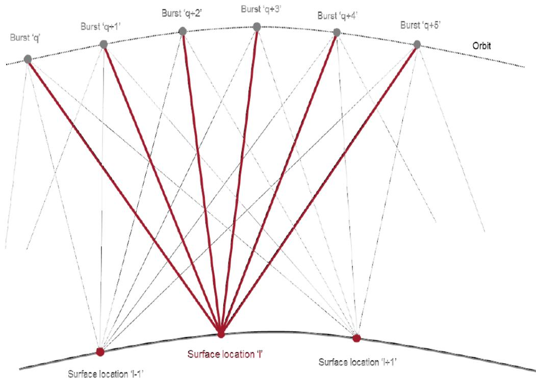
The final height estimate (retracking) is made on the L1b waveform resulting from the **incoherent averaging of waveforms (looks)**, composing the stack, that point a specific surface location (e.g. 6 looks from 6 different bursts are reported in the figure).
