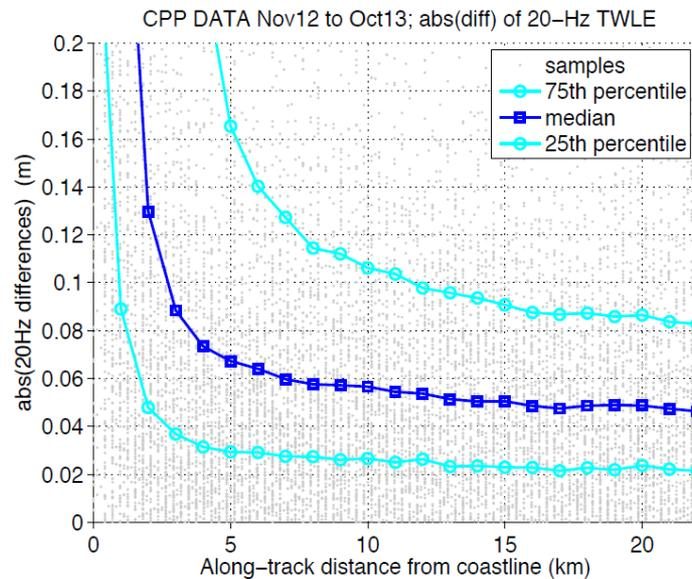
Figure 8: scatterplot of the absolute value difference between consecutive TWLE measurements against **along-track** distance from coast, and the statistics of its distribution in 1-km distance bins, for the CPP dataset.
