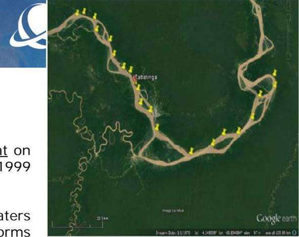
Figure 38: Google earth image of Amazon near Tabatinga. Gauge marked in red. Yellow markers denote centre line of stretch considered for Cryosat-2 crossings.
