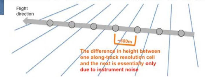
Figure 1: schematics of the use of difference in height between adjacent resolution cells as a proxy for instrumental noise.
