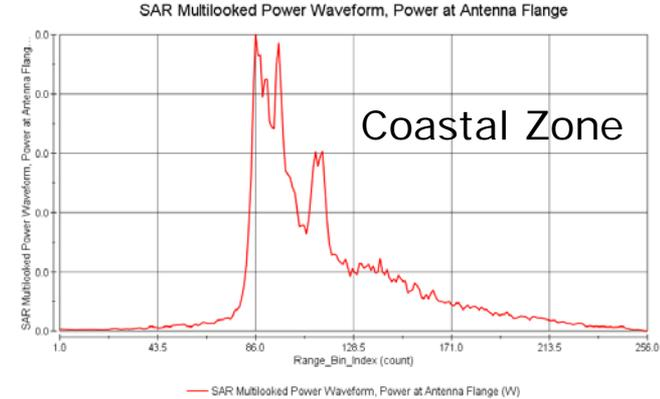
Appended to each record is the **number of looks** used in the averaging and the correspondent Doppler angles identifying the displacement of the looks. **They are needed to support the retracking phase** (only analytical retracking). Empirical retrackers do not need any additional information (not an advantage in case of mispointing).
