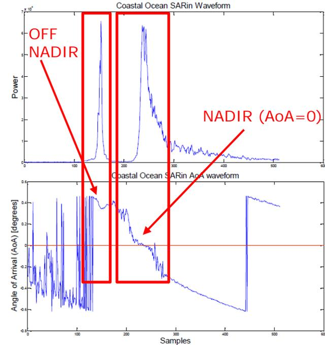
Figure 2-2. Example of a Coastal Ocean contaminated waveform. TOP: Power waveform. BOTTOM: Angle of Arrival waveform.
