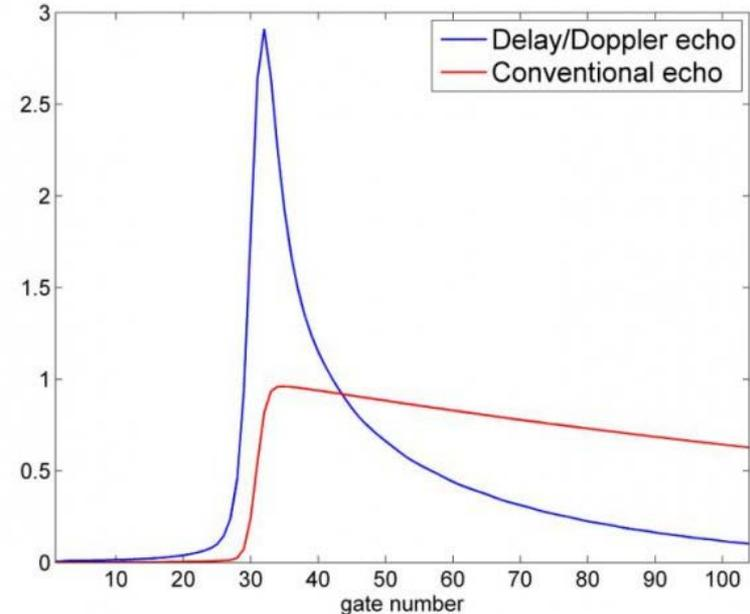
The incoherent averaging (multi-looking) of the individual echoes in the stack leads to a different result, if compared to the incoherent averaging made on LRM altimeters.
