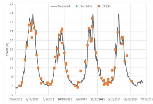
Figure 20: Comparison of Kratie gauge data with heights from near-by altimetric points from NCL (this study) waveforms using N=40. RMS 67.8 cm (empirical retracker) and 66.9 cm (OCOG/Threshold) using 3 $\sigma$  rejection level.
