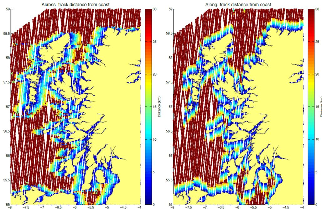
Figure 5: across-track and along-track distance from coast for CryoSat-2 passes around the Western coast of Scotland.
