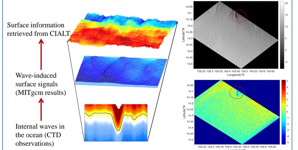
**Figure 6.** The left graph shows the conceptual graph of detection of internal waves using CIALT data. The right graph shows a case study of internal wave using CIALT images (Top figure shows the map of Sigma0 and the bottom figure shows the map of retrieved sea surface height from CIALT data).
