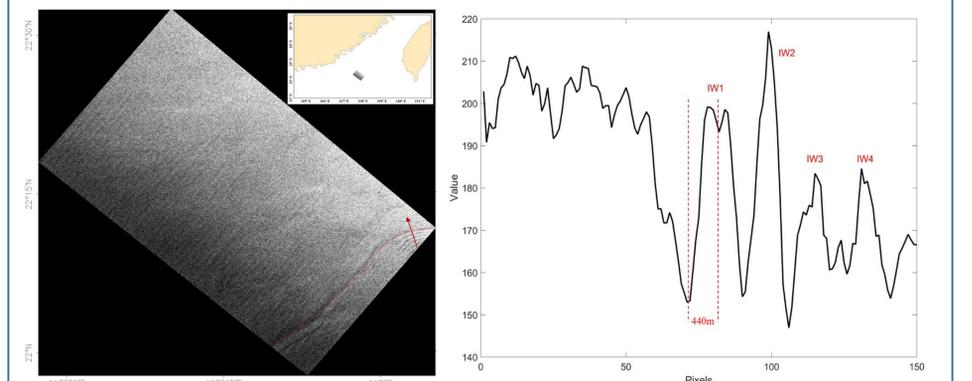
**Figure 7.** Internal wave detection using CIALT image in the SCS (left graph), the propagation direction is 336°. The right graph shows the extracted profile and measured peak to trough distance. The calculated amplitude of leading wave is 61.1m.
