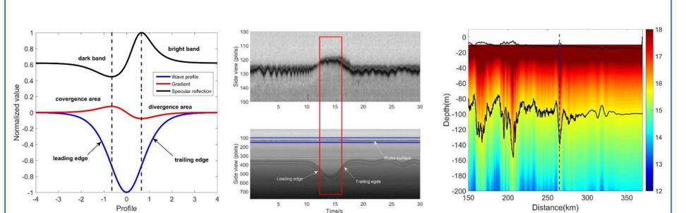
**Figure 5.** Conceptual graph of the opposite-phase relation between the profiles of internal wave and the surface elevation (left graph). The middle graph shows the experiment results and the right graph shows the results of MITgcm.
