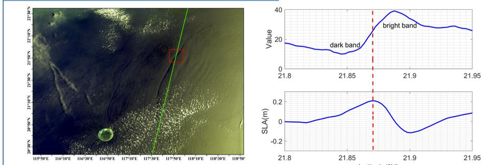
**Figure 4.** Synchronous detection of internal waves in the SCS using OLCI image (right graph) and SAR mode altimetry data. The green line indicates the ground tracks of altimeter. The right graph shows the profile extracted from OLCI image and SSHA of SRAL records.
