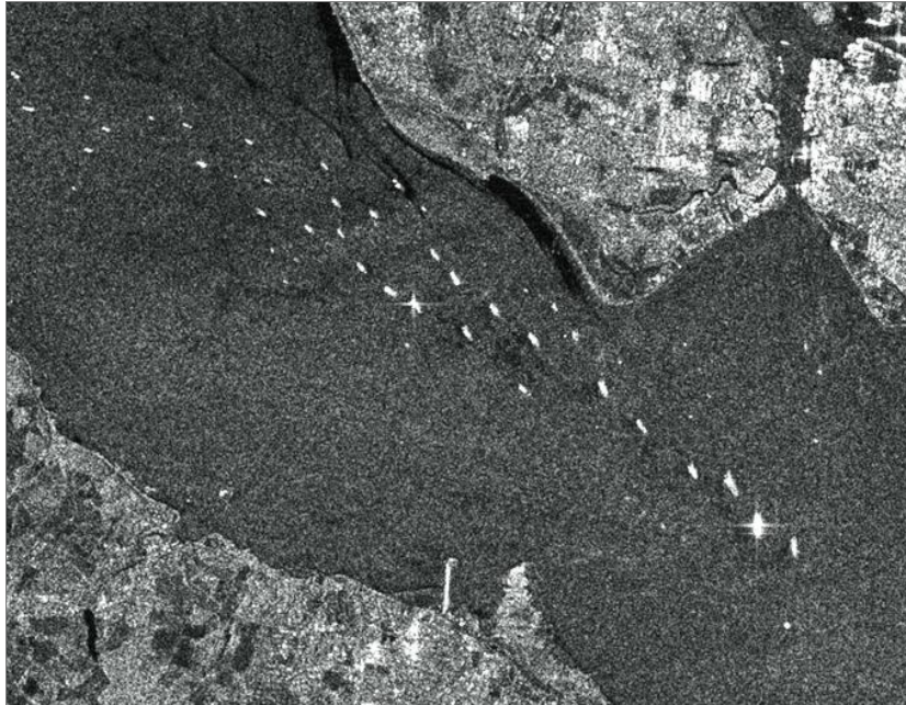
Figure 2: ASAR Image Showing the Ships for the International Fleet Review Assembling in the Solent Between the Isle of Wight and Portsmouth on June 26th 2005.
