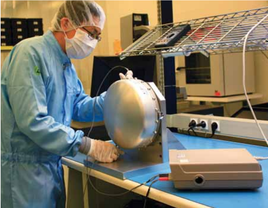
Figure 4.3. Reaction wheels. (Bradford Engineering, the Netherlands)
