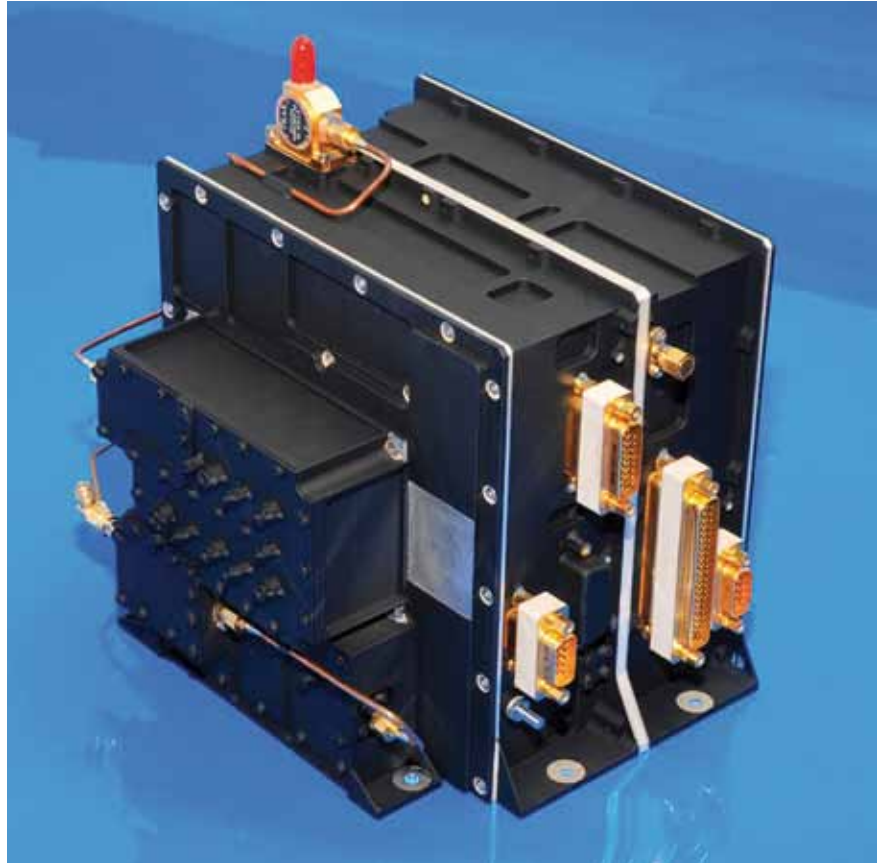
Figure 4.11. S-band transponder. (Thales Spain)
