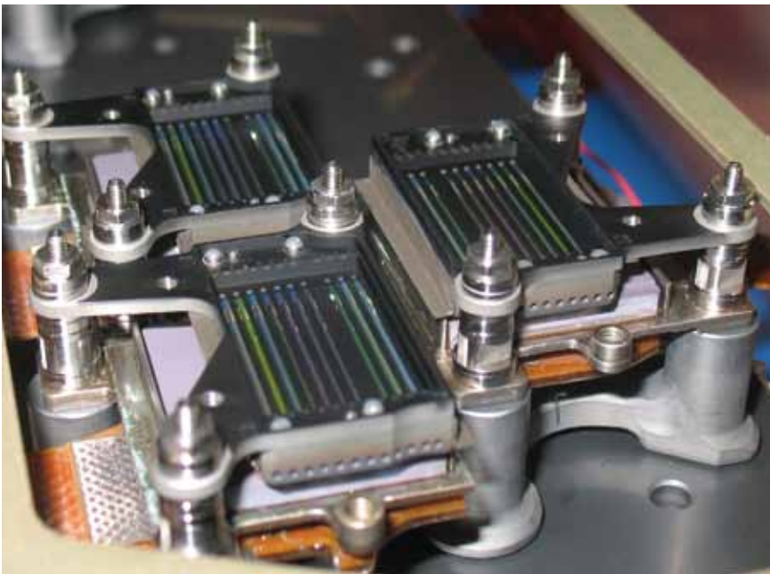
Figure 4.20. VNIR filter assemblies positioned on top of the detectors on the FPA. The assembly design and materials have been optimised to minimise straylight. (Jena-Optronik, Germany)
