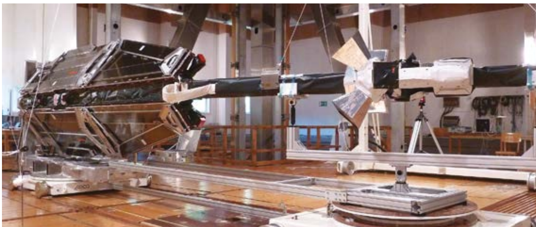
One of the Swarm satellites, with boom deployed, undergoing tests at IABG's Magnetic Field Simulation Facility in Germany. The tests are carried out in a magnetically clean environment, hence the wooden floor. (ESA/IABG)
