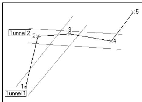
Fig. 1: Tunneling: The first tunnel is constructed around node 1, and intermediate coordinates 2 and 3. Intermediate coordinate 2 falls outside the tunnel and thus remains. The second tunnel is constructed around intermediate coordinates 2, 3, and 4. Intermediate coordinate 3 falls inside the tunnel and is thus omitted. Now that point 3 is omitted, the next tunnel will be constructed around intermediate coordinates 4, 5, and 6 (point 6 is not in this picture).
