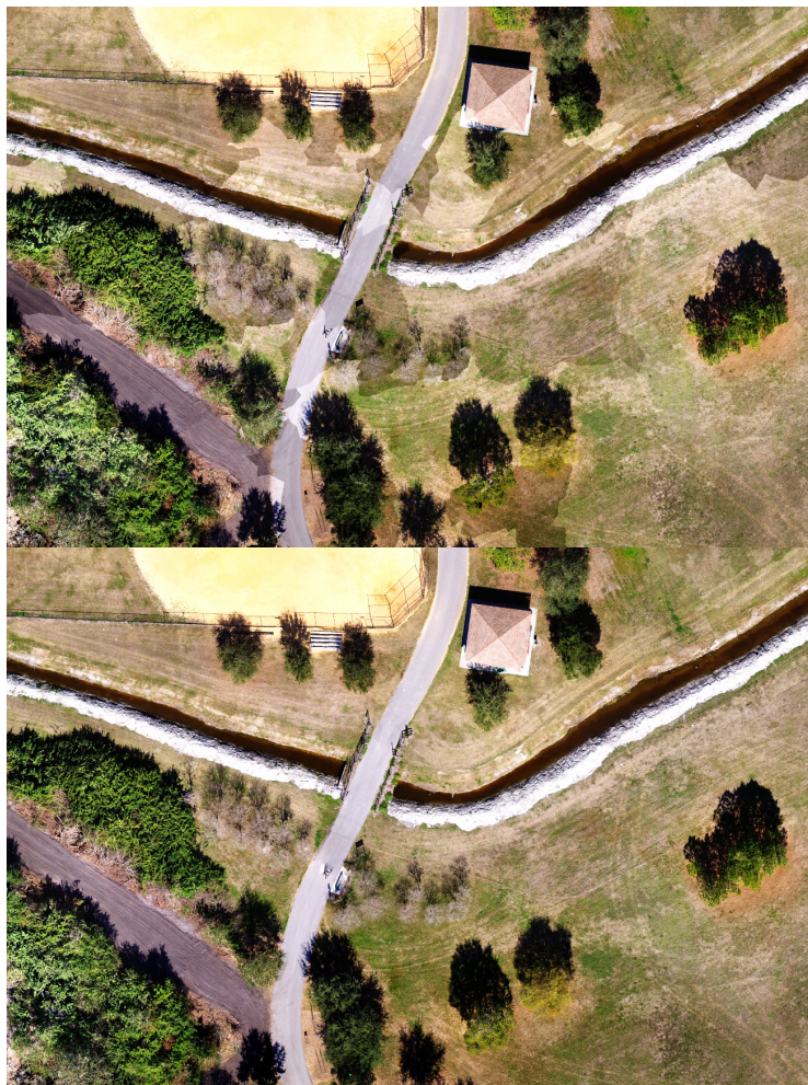
Seams in the textured model due to different light intensities (top) and global seam leveling applied (bottom)
