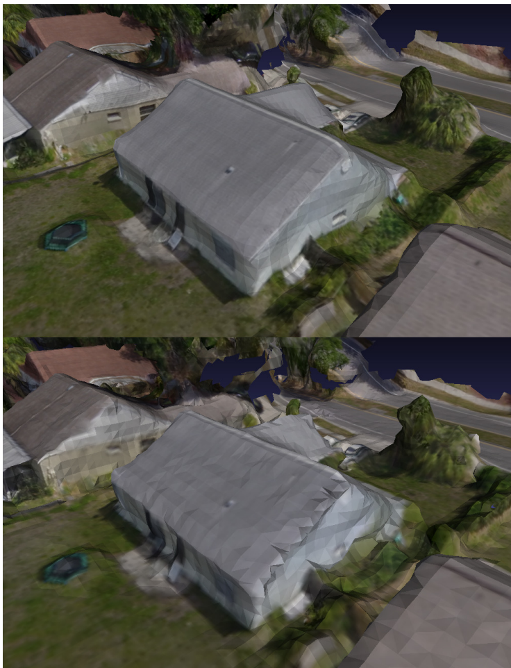
mesh-samples set to 1 (top) 20 (bottom). Ideal values for this option are between 1 and 20
