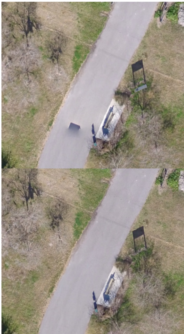
Gauss Damping (top) vs. Gauss Clamping (bottom). Note a part of the cart was missed in the top image
