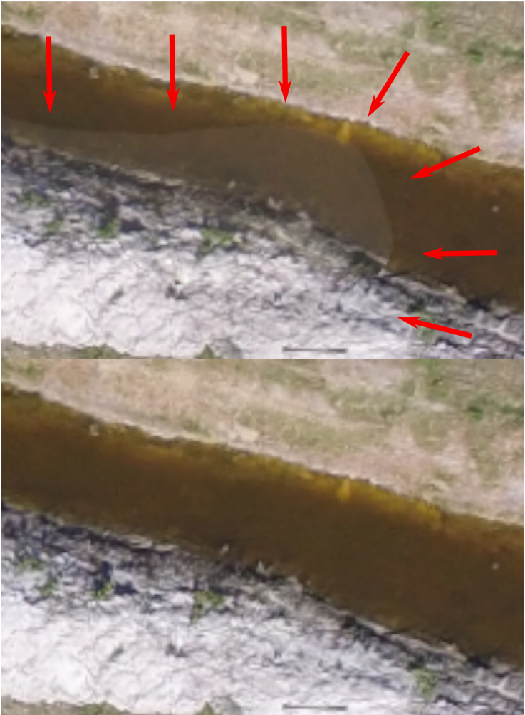
Result with global seam leveling, but not local seam leveling (top) and with local seam leveling (bottom)
