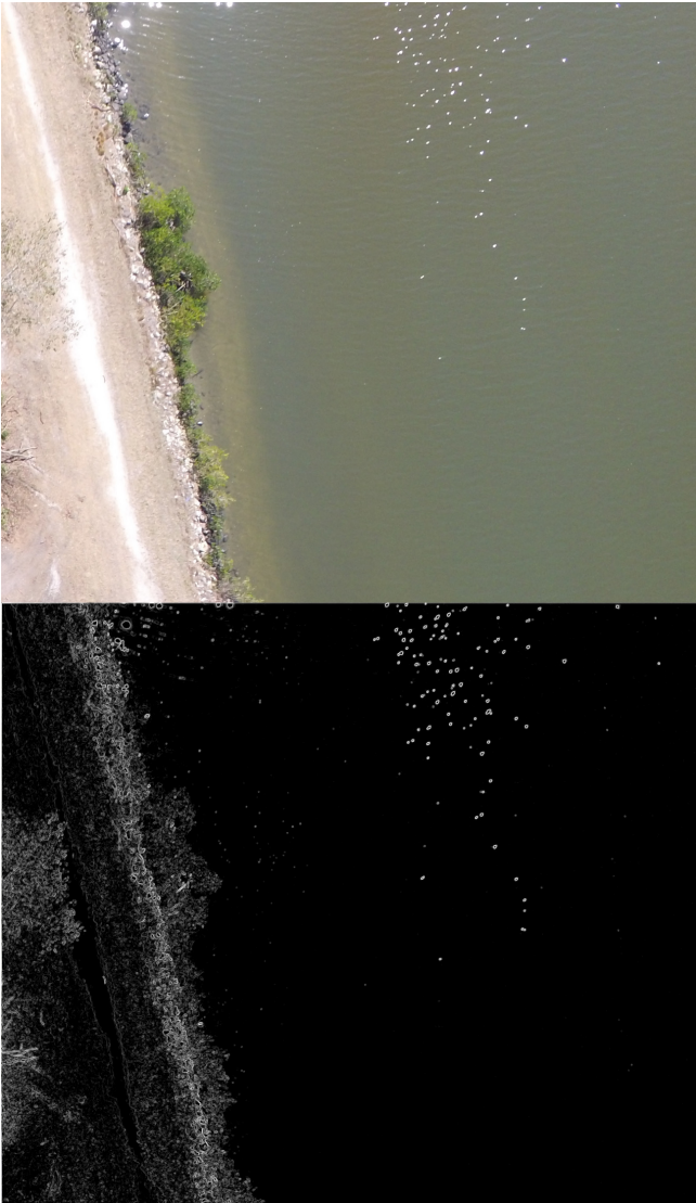
An image (top) vs. Sobel edge detector mapped to a black-white gradient (bottom). The water shows small changes in gradient, whereas the shoreline has a higher gradient magnitude
