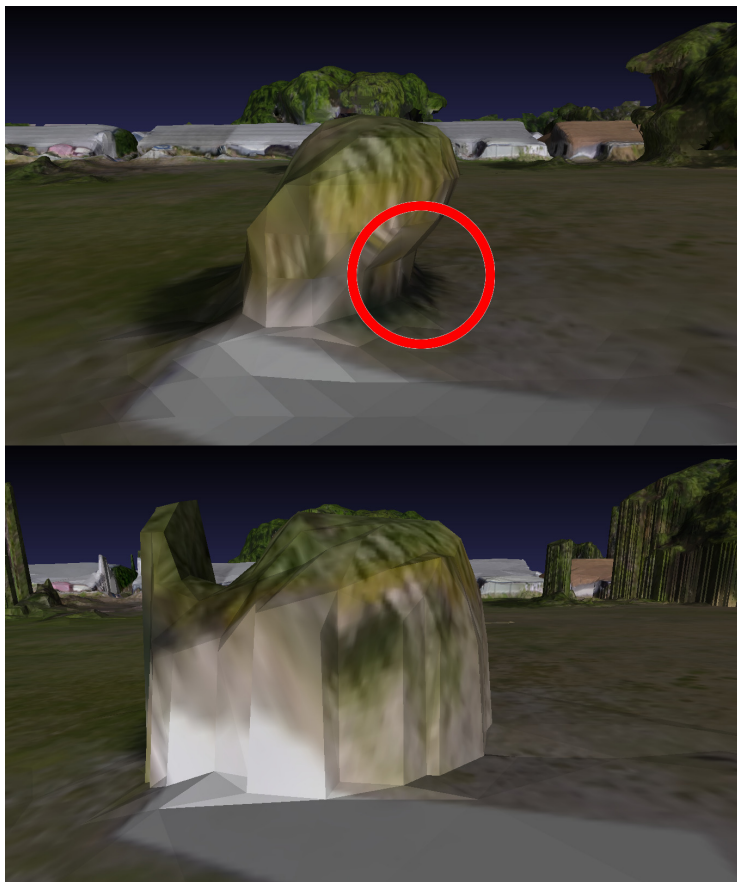
3D model (top) vs. 2.5D model (bottom). Note the absence of overhangs on the bottom
