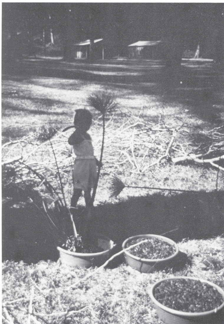
Fig. 12. Photo showing the 'meteorological site' used for observations in Oct. 1986 at Fisherman's camp. The two Salvinia -pans appear in the foreground together with the papyrus-pan. The child is holding a papyrus -stalk used for the studies of transpiration. Photo: L.E. Åse.
