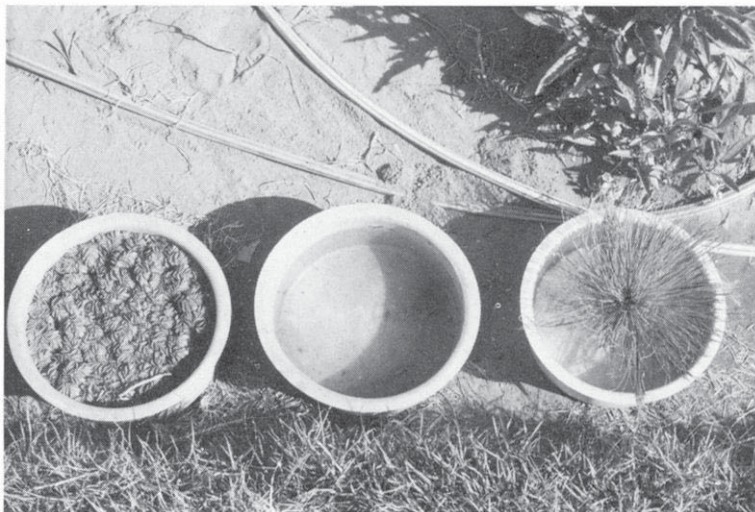
Fig. 9. Photo showing the pans used for the studies of evaporation, transpiration and water uptake. (Cf. text and Fig. 11). Photo: N. Tarras-Wahlberg.
