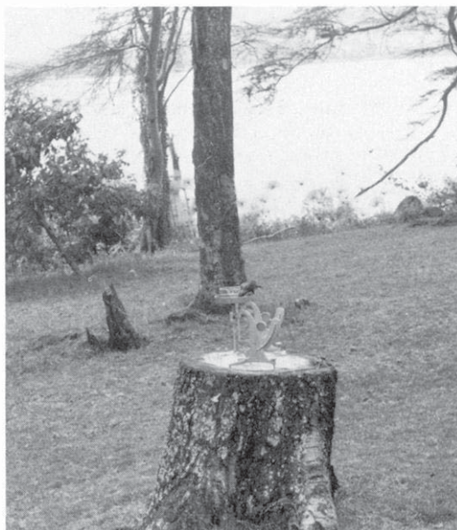
Fig. 10. Photo showing the balances used for studies of evapotranspiration from Salvinia . Photo: N. Tarras-Wahlberg.
