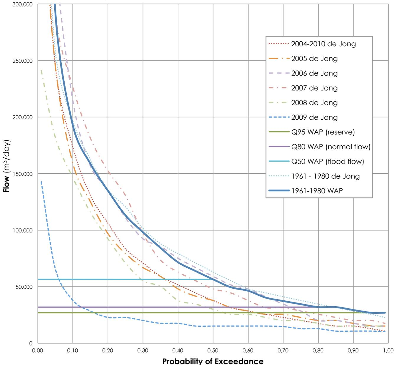
Figure 13: 2GB4 WAP and newly composed (de Jong, Source WRMA) FDCs and regulative flow thresholds (Q-Flows).
