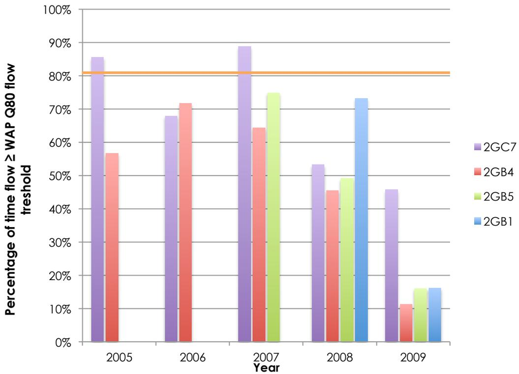
Figure 17: Percentage of time river flow equals or exceeds the WAP Q80 flow at the stations 2GB1, 2GB4, 2GB5, 2GC7
