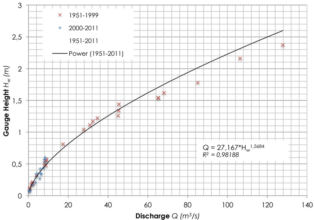
Figure 7: Rating curve showing the relationship between the gauge height and discharge at the 2GB1 gauging station in the Malewa River (x and + markers represent a flow measurement Source: WRMA / MWI)
