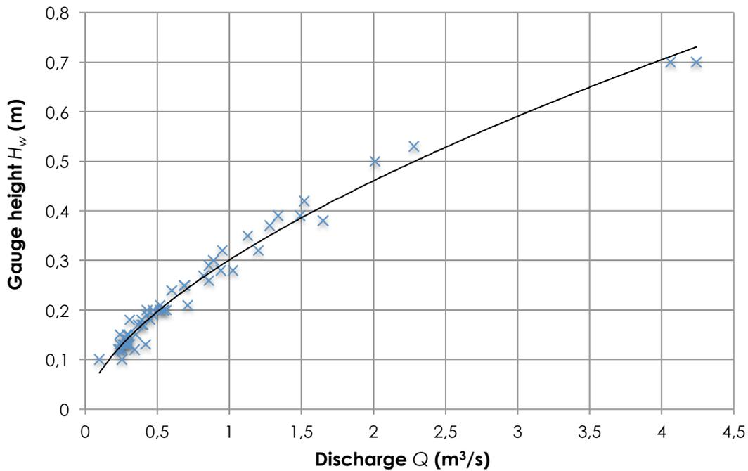
Figure 4: Example Rating Curve
