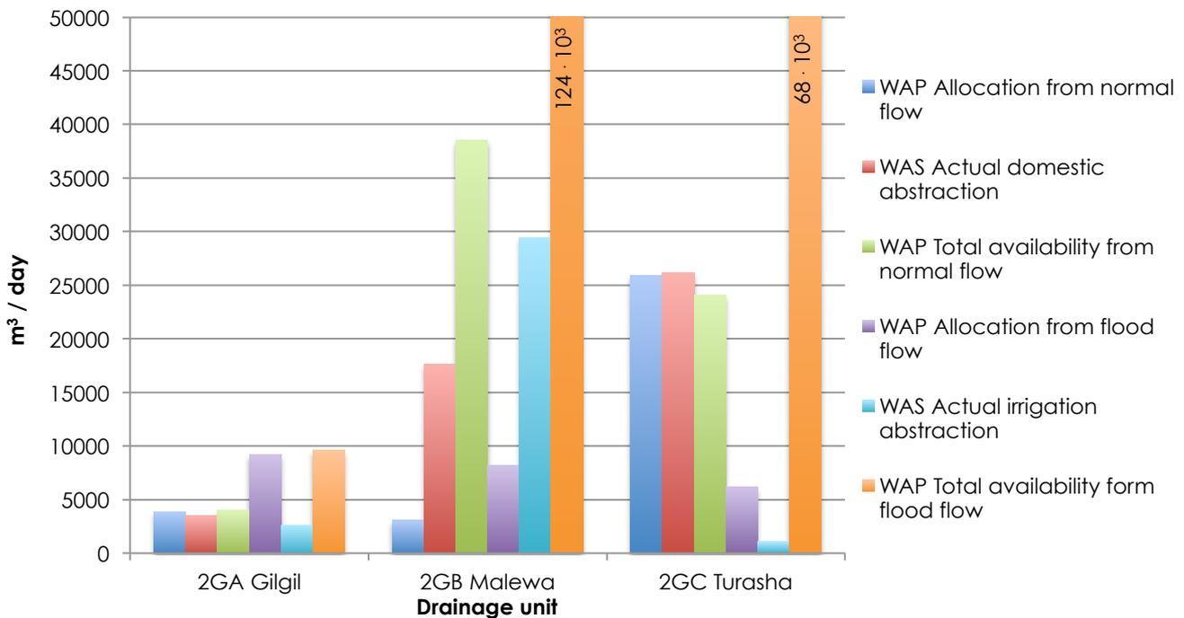
Figure 19: River water abstraction data compared to the allocation and availability as indicated by the WAP for normal and flood flow (Jong, 2011).
