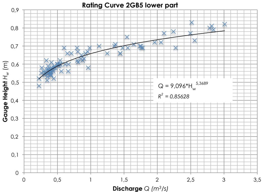
Figure 9: Rating curve showing the relationship between the gauge height and discharge at the 2GB5 gauging station in the Malewa River for the low-end discharges (x markers represent a flow measurement Source: WRMA/MWI)
