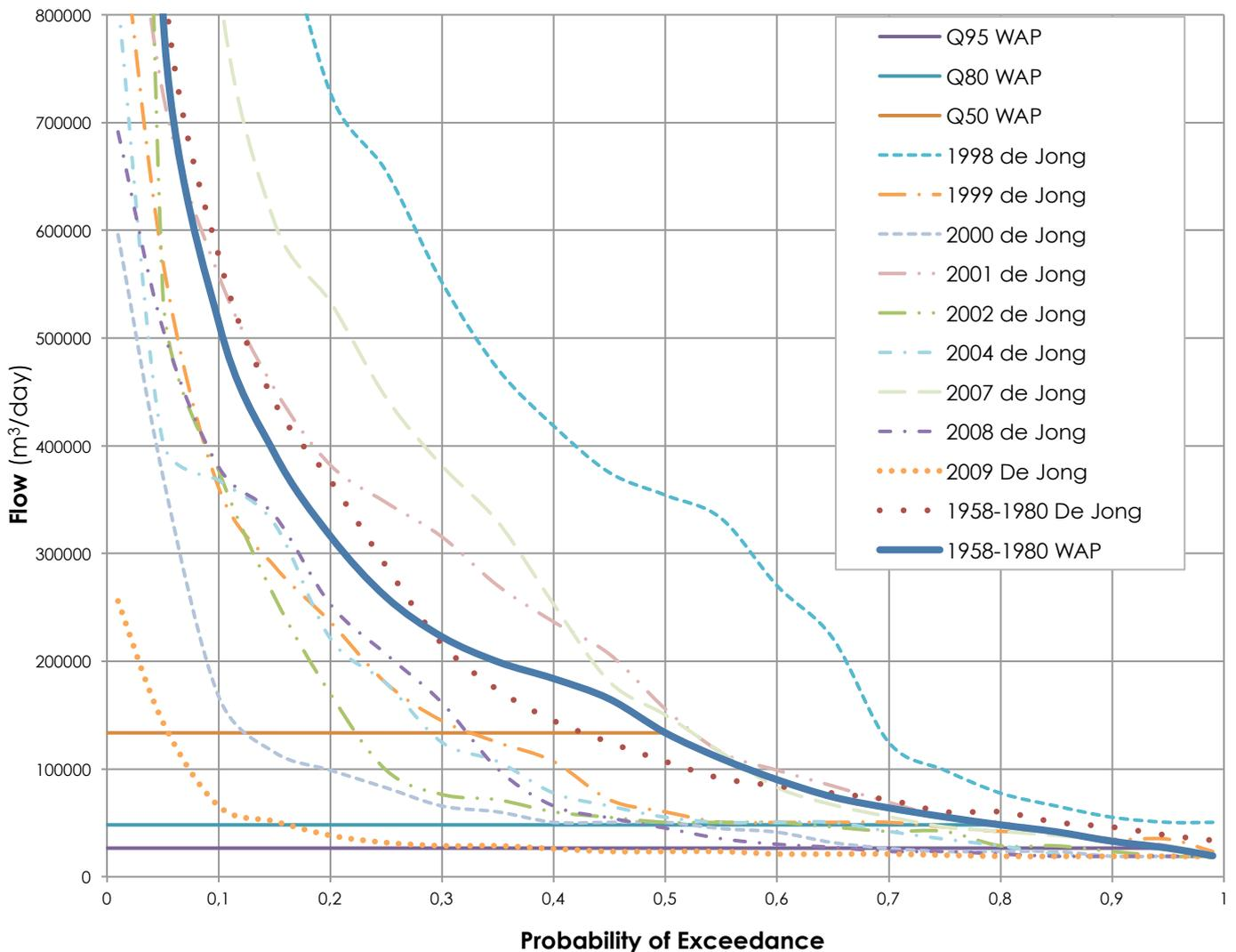
Figure 14: 2GB5 WAP and newly composed (de Jong, Source WRMA) FDCs and regulative flow thresholds (Q-Flows).
