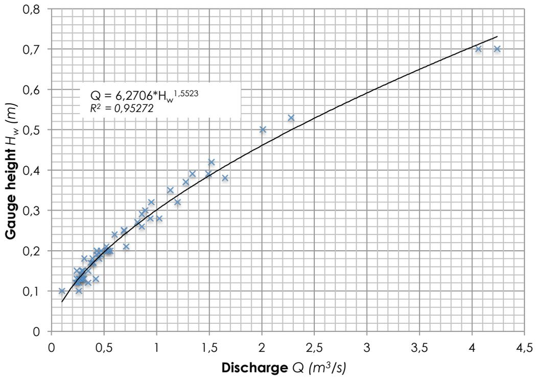
Figure 8: Rating curve showing the relationship between the gauge height and discharge at the 2GB4 gauging station in the Wanjohi River (x markers represent a flow measurement Source: WRMA/MWI)
