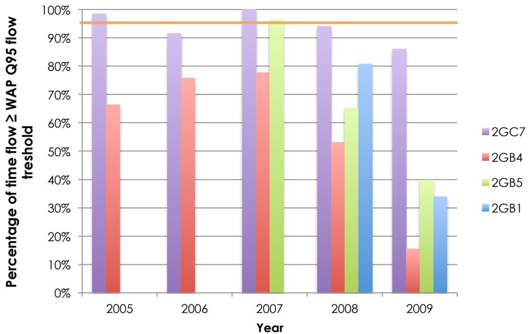
Figure 18: Percentage of time river flow equals or exceeds the WAP Q95 flow at the stations 2GB1, 2GB4, 2GB5, 2GC7
