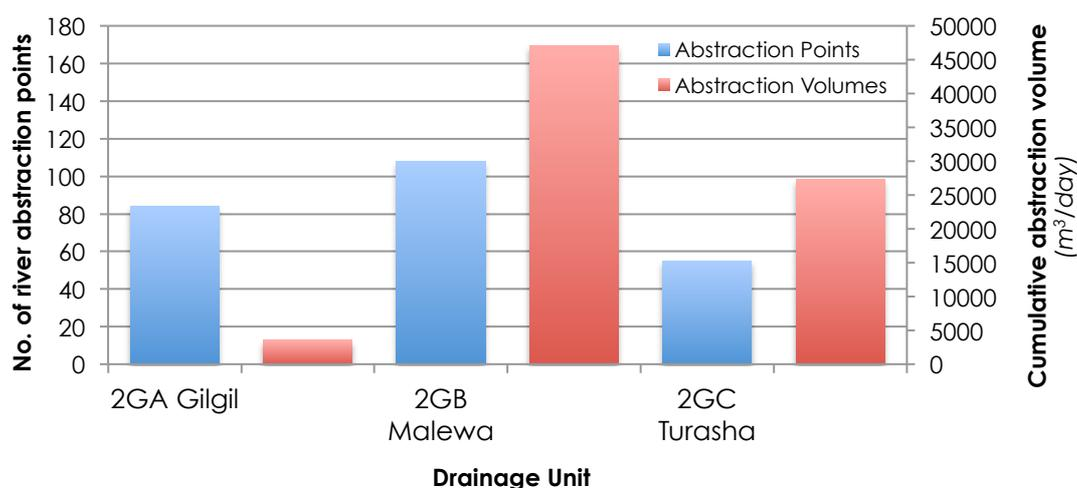
Figure 6: Comparing river abstraction- points and volumes between the different drainage units (Jong, 2011)
