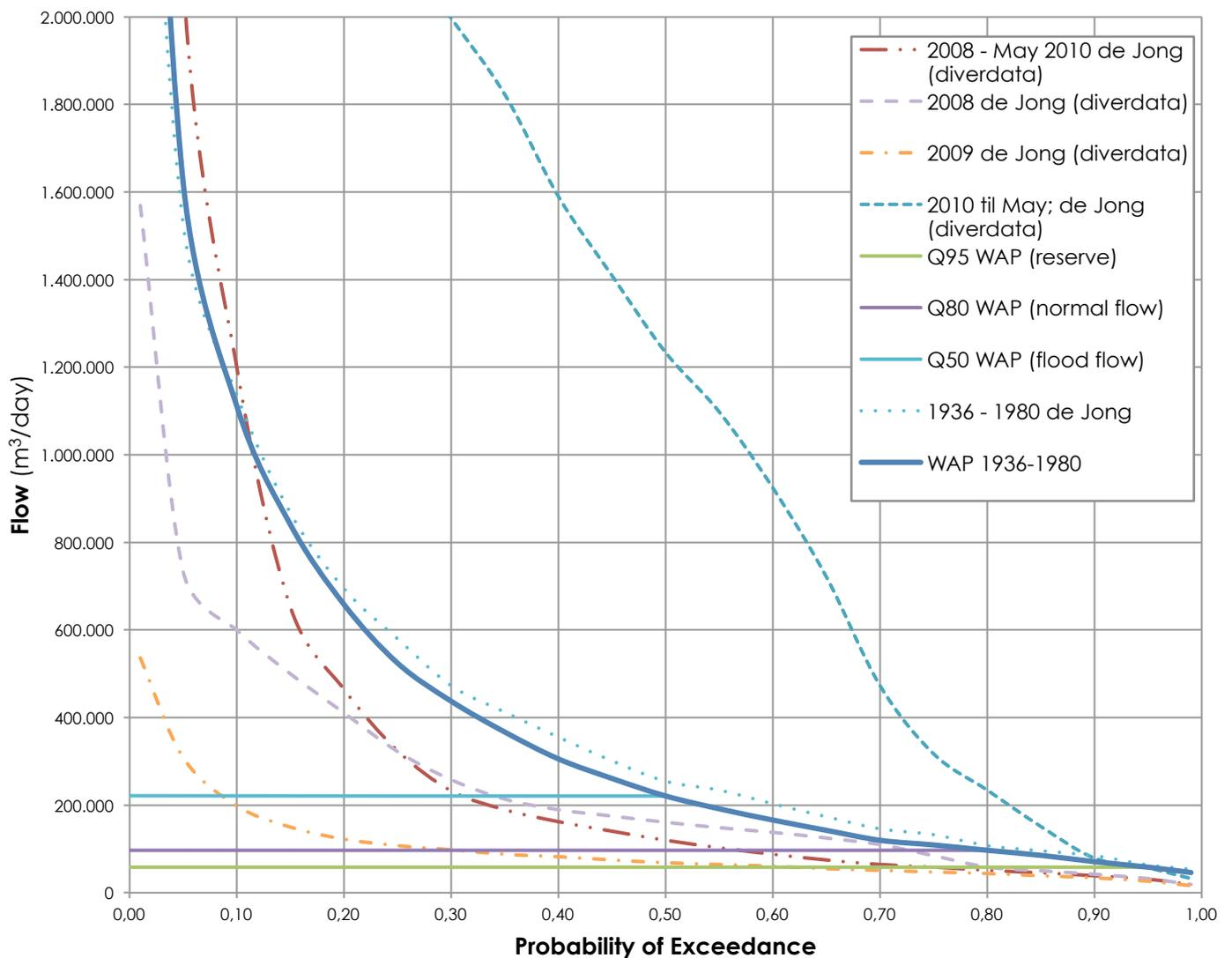
Figure 12: 2GB1 WAP and newly composed (de Jong, Source WRMA) FDCs and regulative flow thresholds (Q-Flows).
