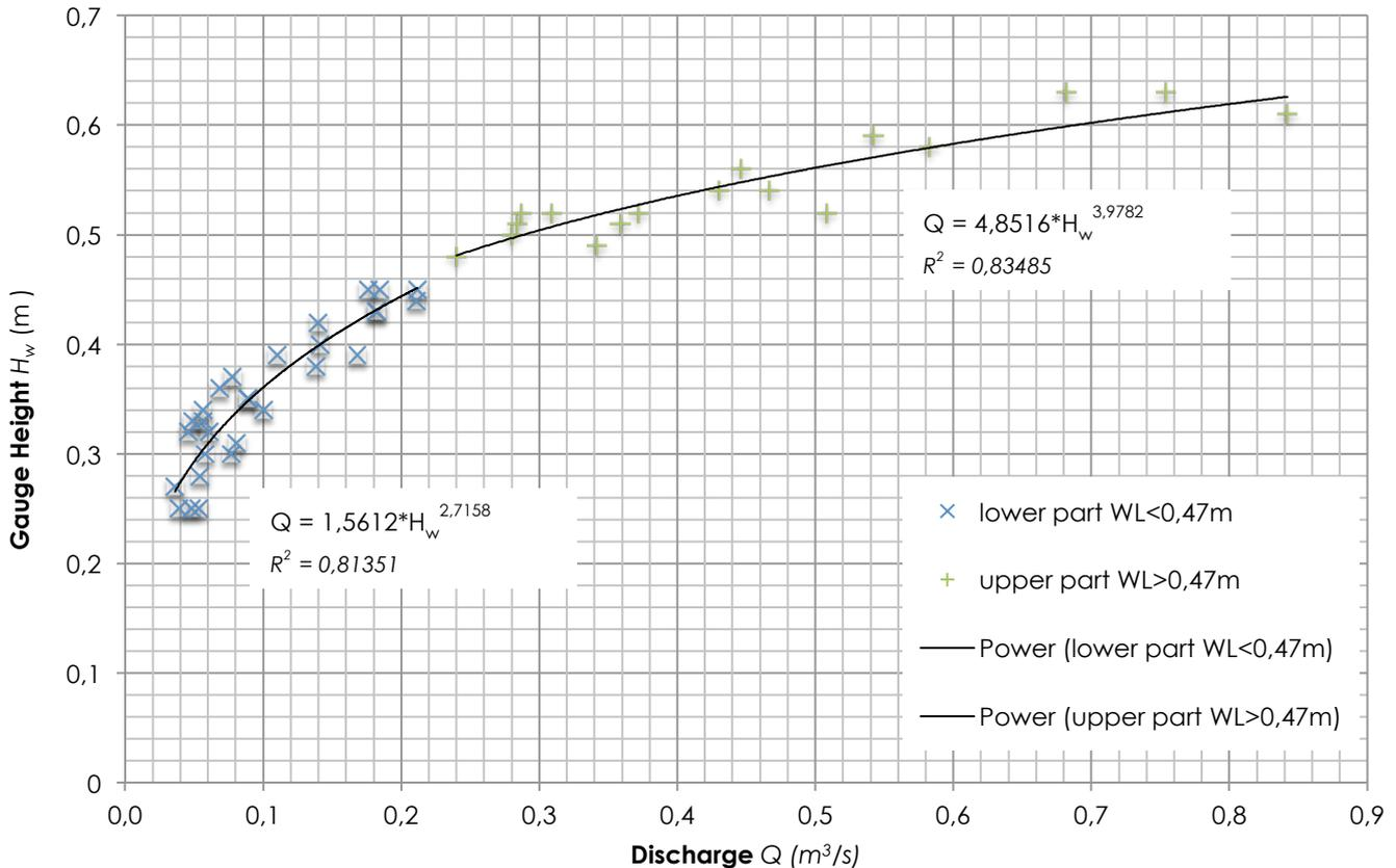
Figure 11: Rating curves showing the relationship between the gauge height and discharge at the 2GC7 gauging station in the Turasha River (x and + markers represent a flow measurement Source: WRMA/MWI)
