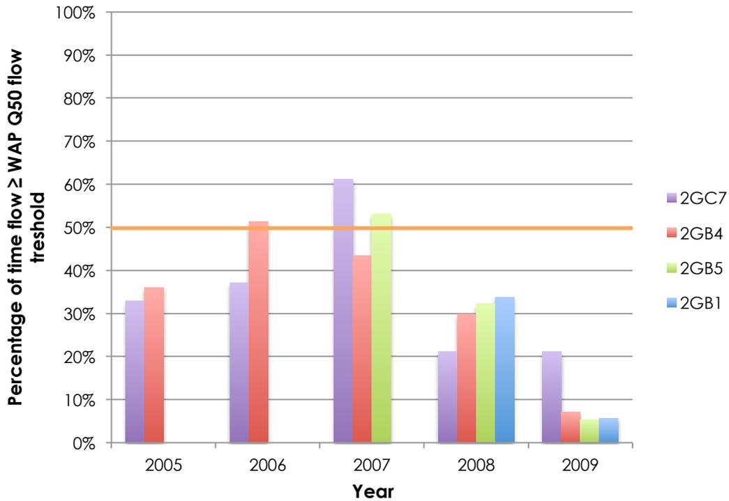
Figure 16: Percentage of time river flow equals or exceeds the WAP Q50 flow at the stations 2GB1, 2GB4, 2GB5, 2GC7
