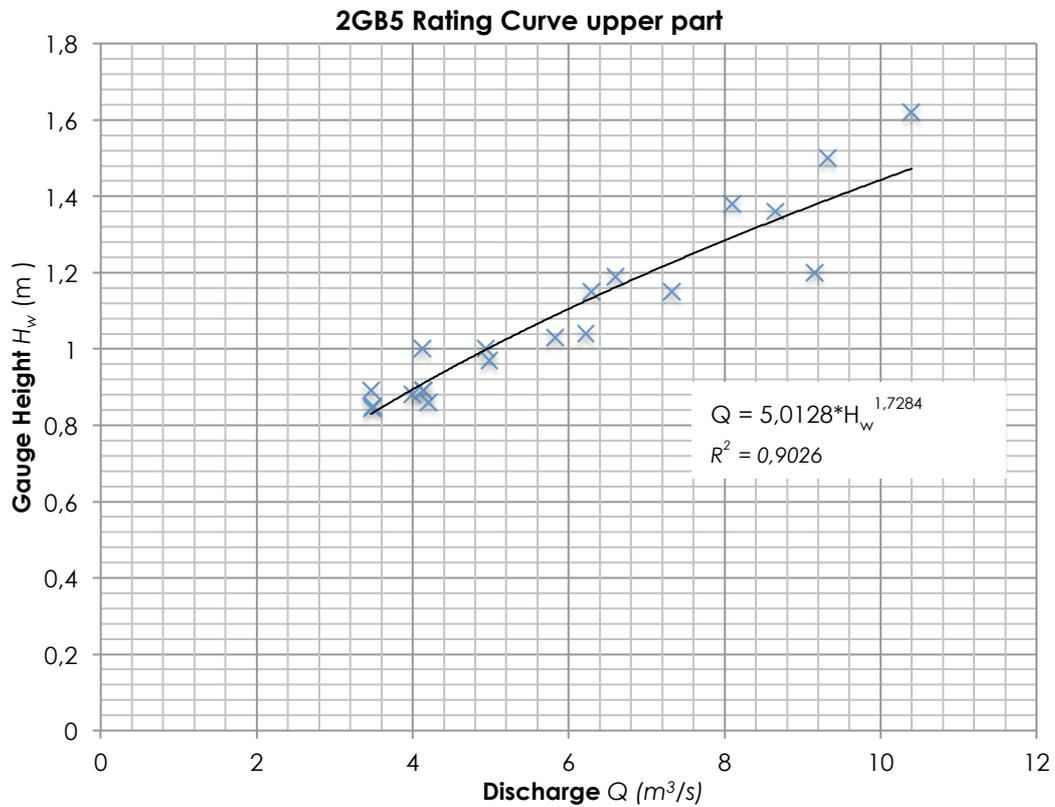
Figure 10: Rating curve showing the relationship between the gauge height and discharge at the 2GB5 gauging station in the Malewa River for the high-end discharges (x markers represent a flow measurement Source: WRMA/MWI)
