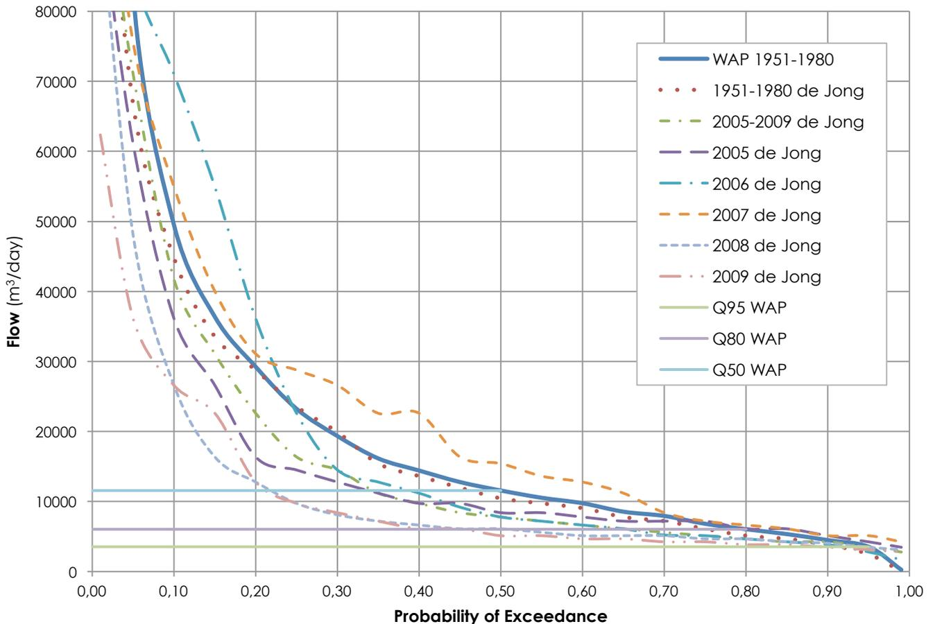
Figure 15: 2GC7 WAP and newly composed (de Jong, Source WRMA) FDCs and regulative flow thresholds (Q-Flows).
