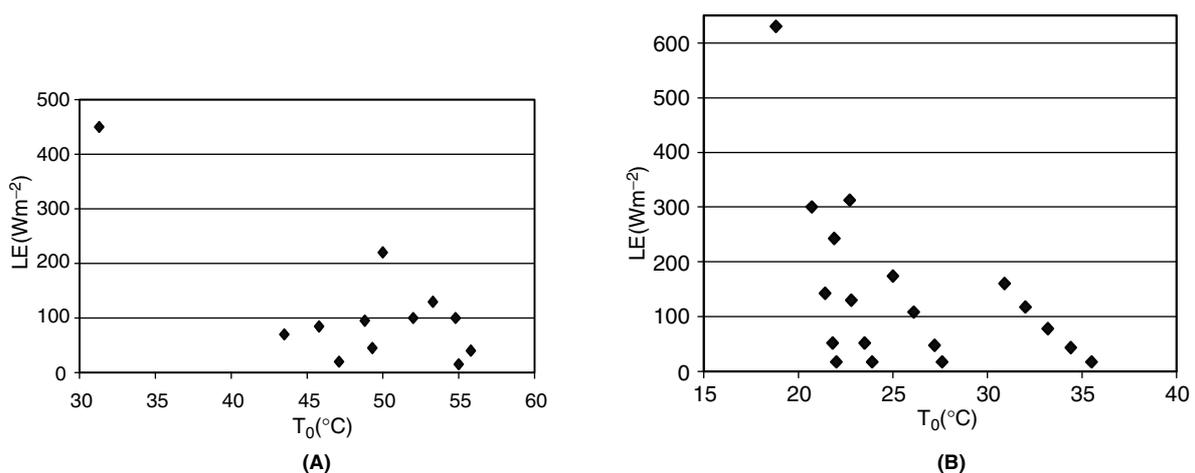
Figure 1. Latent heat flux as a function of surface temperature. (A) Field measurements in Castilla la Mancha (Pelgrum and Bastiaansen, 1997). (B) Model simulation in a patchy landscape with intermittent wet and dry surfaces (Blyth, 1994)
