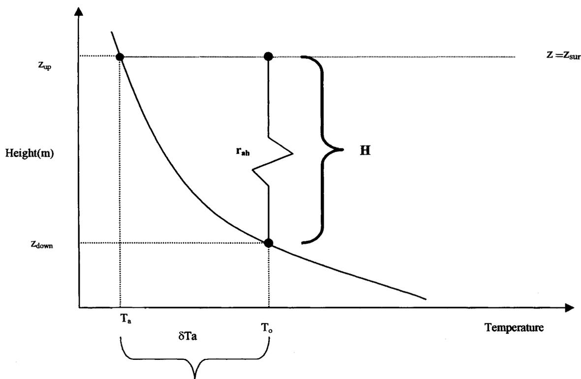
Figure 2. Theoretical profiles of air temperature ( $T_a$ ) in relation to integration limits ( $z_{down}$  and  $z_{up}$ ) affecting the aerodynamic resistance to heat transport ( $r_{ah}$ ) and the radiometric surface temperature ( $T_0$ )
