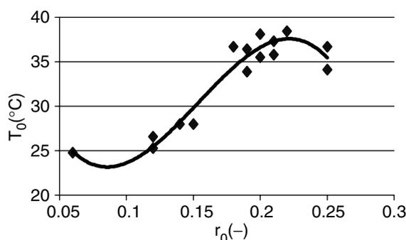
Figure 6. Relationship between surface temperature ( $T_0$ ) and surface albedo ( $r_0$ )
