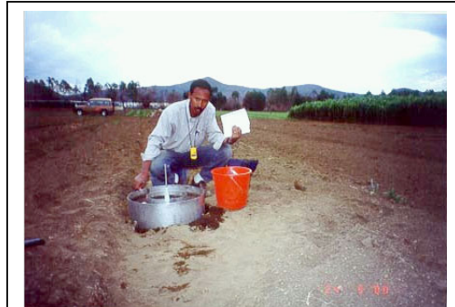
Infiltration test using double ring infiltrometer, Sulmac farm
