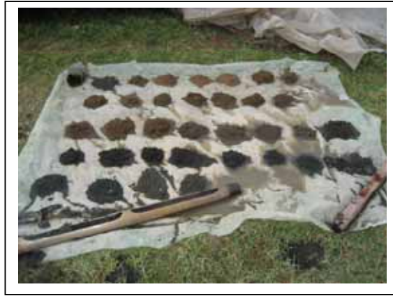
Figure 4-1 Core samples taken from the borehole
