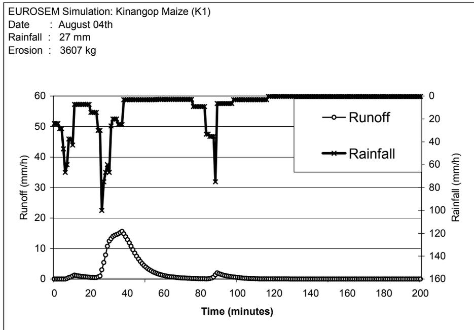
Figure 4-4: Rainfall and runoff simulated by EUROSEM for 27mm rain storm on 4<sup>th</sup> August
