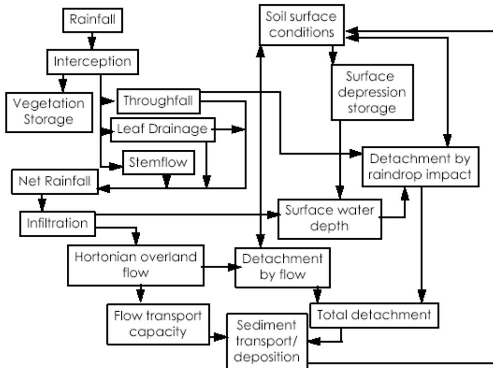
**Figure 2-2: Flow chart for the European Soil Erosion Model (after Morgan et al., 1998)**
