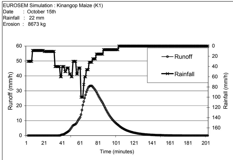
**Figure 4-5: Rainfall and runoff simulated by EUROSEM for 22mm rain storm on 15th October**
