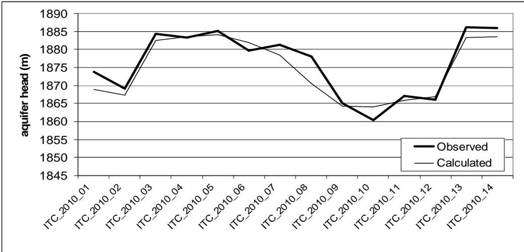
Figure 6:4 Observed and calculated aquifer head (Observation, Jun, 2010)
