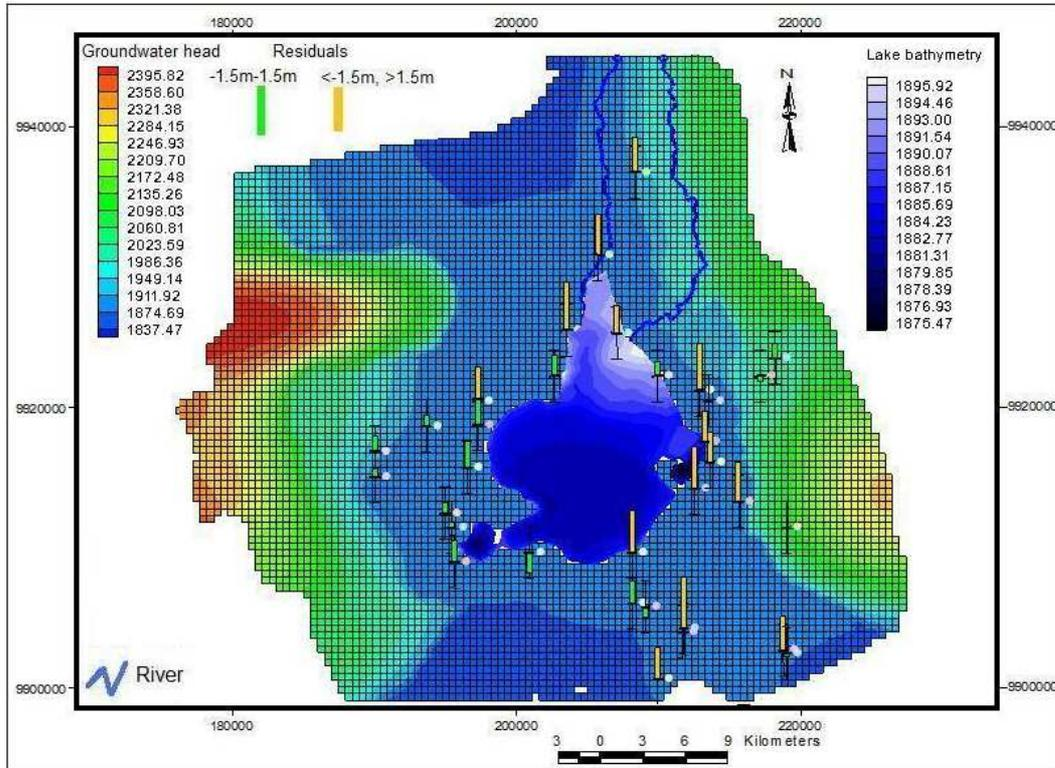
Figure 6:2 Contour map of simulated aquifer heads
