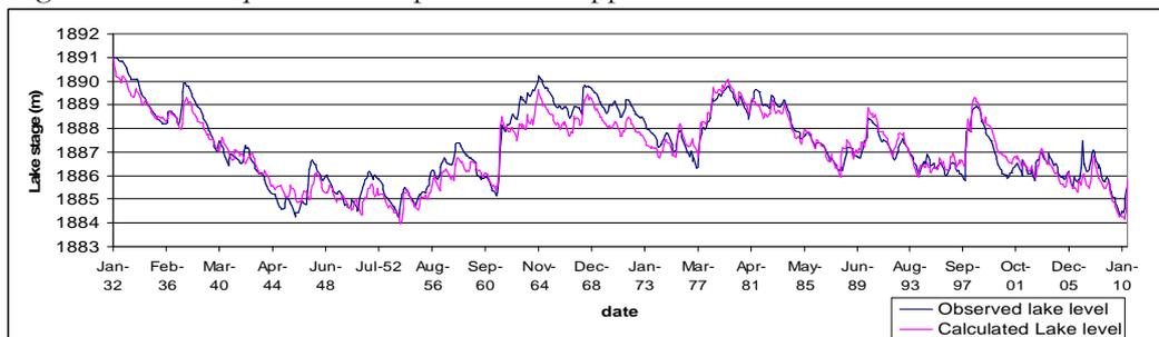
Figure 6:3 Time series plot of observed and calculated lake levels (1932 to 2010)
