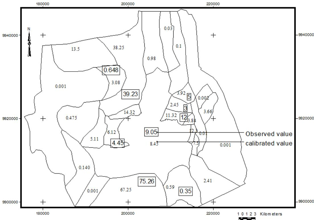
Figure 5:5 Parameter zones for Hydraulic conductivity (layer: 1)
