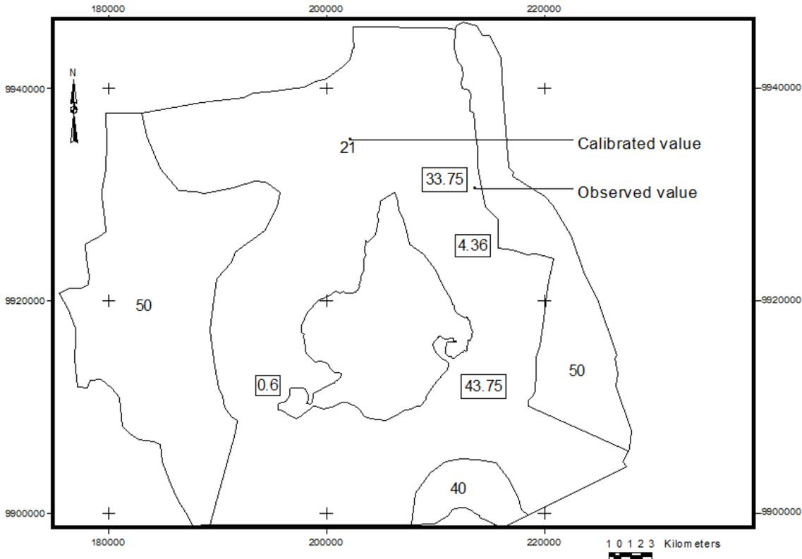
Figure 5:6 Parameter zones for recharge (layer: 1)
