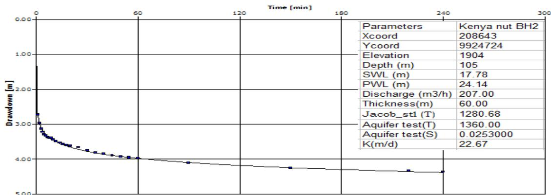
Figure 4:10 Pump test analysis result using aquifer test method
