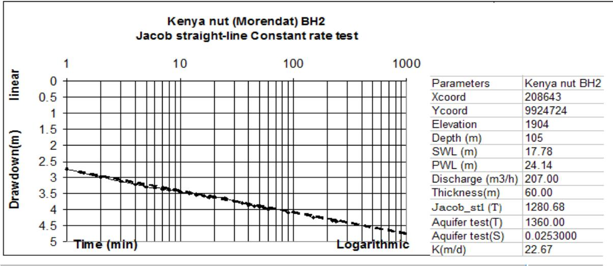
Figure 4:9 Pump test analysis result using Jacob straight-line method
