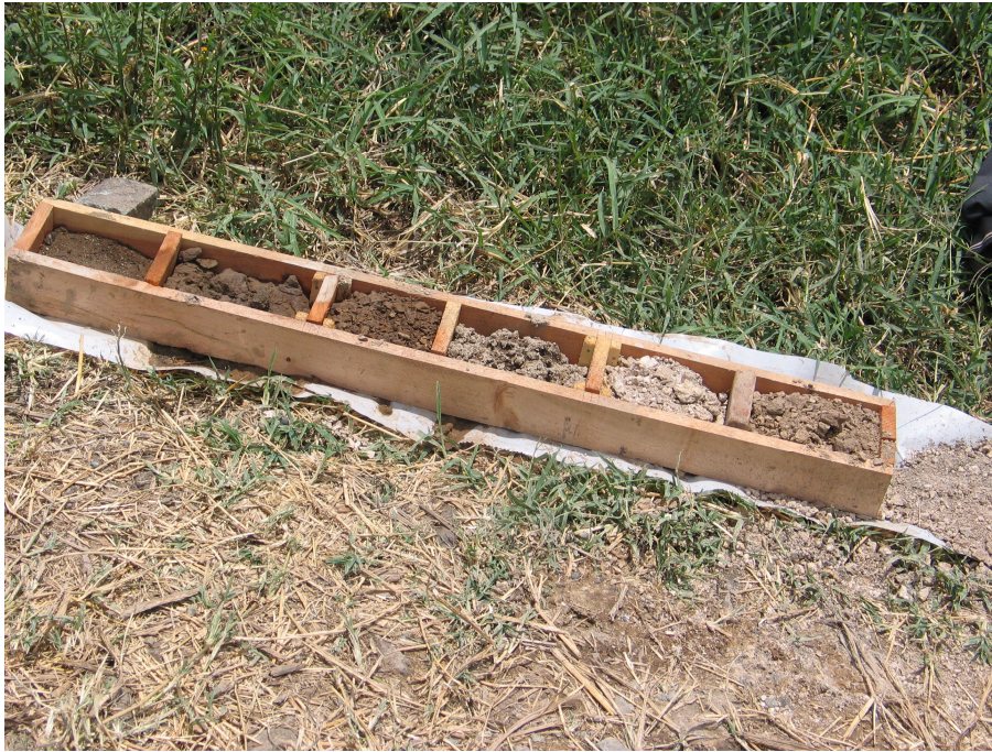
Figure 4.2 Core samples taken from TBH6 at every 5m
