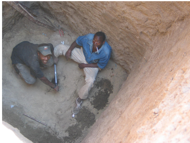
Test pit and auguring
