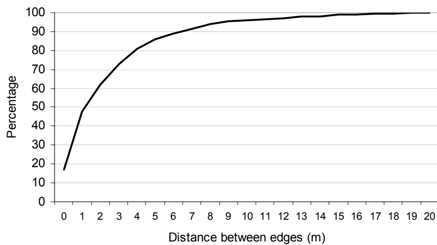
Figure 5. Classification of the distances between edges of SFAP's, georeferenced with direct linear transformation and projective transformation
