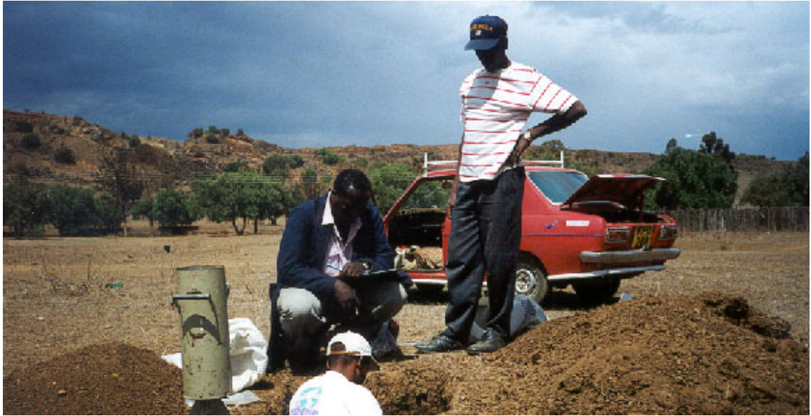
Photo 5. Taking samples for compaction test –sand replacement method(observation point MP-07
