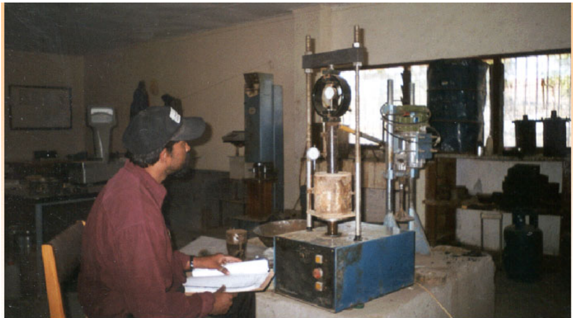
Photo 6. CBR Test on compact soil samples (Soil Engineering Laboratory, Road Maintains Unit, Ministry of Public Works, Naivasha, Kenya
