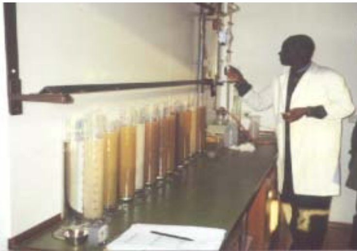
Particle size determination using the pipette method, ITC lab.
