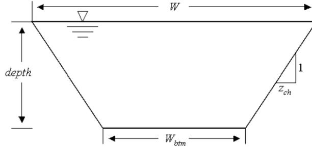
Figure B - 1: Trapezoidal profile used by SWAT
