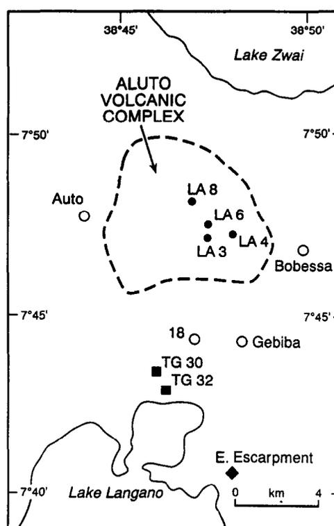
Figure 9. Map of the Aluto-Langano volcanic complex, Ethiopia, situated between Lakes Zwai and Langano, showing the location of geothermal wells, temperature gradient boreholes, fumaroles and cool spring sampling sites.
