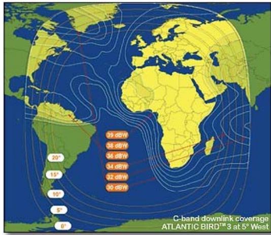
EUTELSAT 5 WEST C-band system setup dBW footprint
