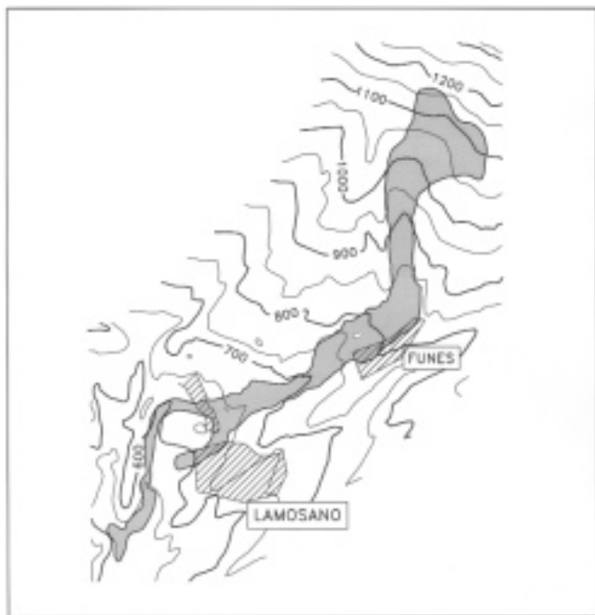
FIGURE 6: Prediction of a future scenario due to remobilization of about 1 million m 3 of material.
