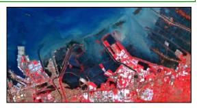
Figure 3.C.22-B: A Subsidence flooding in the industrial area of Semarang city, Indonesia. Asterbands RGB: 321 (M. Damen, 2009)
