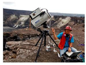
Figure 3.V.10: Fourier Transform Infrared Spectrometer (FTIR) deployed at a volcano.
