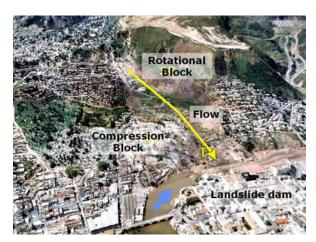
Figure 1.15: Overview of the hazard event with a landslide that dammed the river. Source: R. Peñalba
