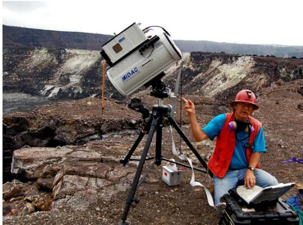
*Figure 3.V.10: Fourier Transform Infrared Spectrometer (FTIR) deployed at a volcano.*
