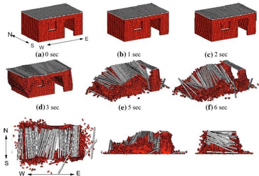
Figure 5.15: Example of a numerical simulation of a masonry building under an earthquake, comparable to the Bam earthquake (Source: Furukawa and Ohta, 2009)
