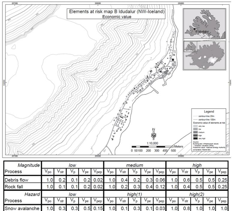
Figure 5.16: Vulnerability study in Iceland. V<sub>po</sub> = vulnerability of a power line, V<sub>str</sub> = vulnerability of roads and infrastructures, V<sub>p</sub> = vulnerability of properties (buildings), V<sub>pe</sub> = vulnerability of people and V<sub>pep</sub> = vulnerability of people in buildings. Source: Bell and Glade 2003)
