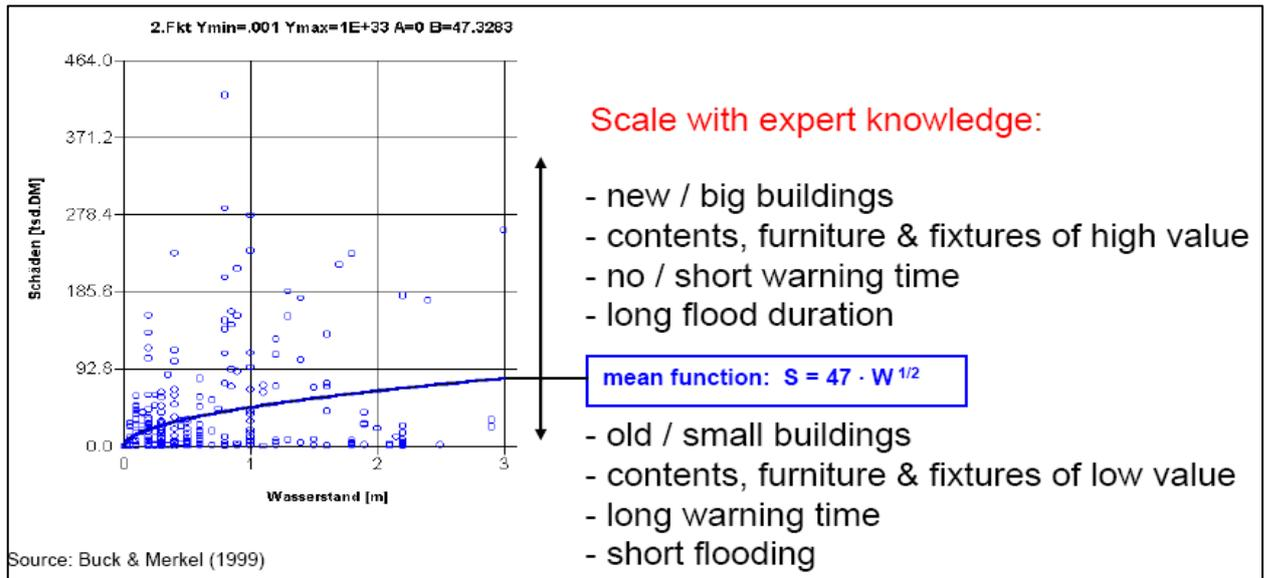
Figure 5.13 Example for a damage function from the HOWAS database.
