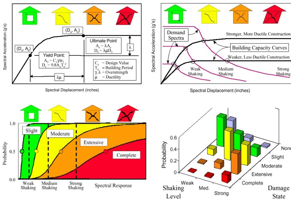
Figure 5.18: HAZUS method for earthquake loss estimation of buildings.
