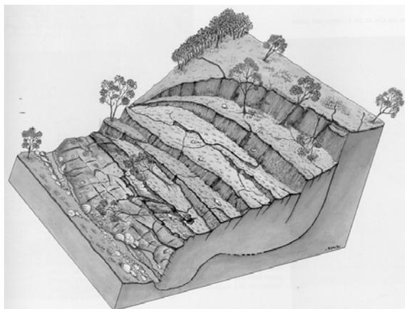
Figure 2.4: Block diagram of a rotational slide
