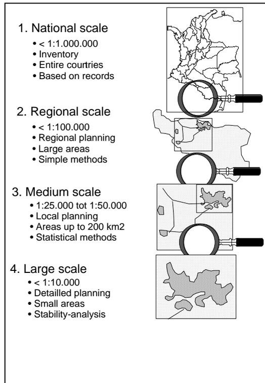
Figure 3: Scale of landslide hazard zonation, objectives and general approaches.
