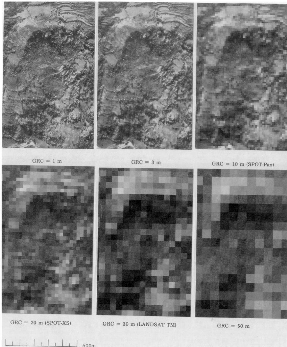
Figure ? : An area showing a landslide scar that is in shadow (high contrast) in the central upper part of the picture and a depositional area of landslide debris (low contrast) in the central to lower part of the picture. The pictures were show how the same landslide would be displayed on aerial photos , SPOT Pan, SPOT XS, and LANDSAT TM
