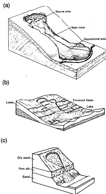
Figure 2.6: Examples of flows: a: slow earth flow, B: Loess flow, c:dry sand flow (Cruden and Varnes, 1996)
