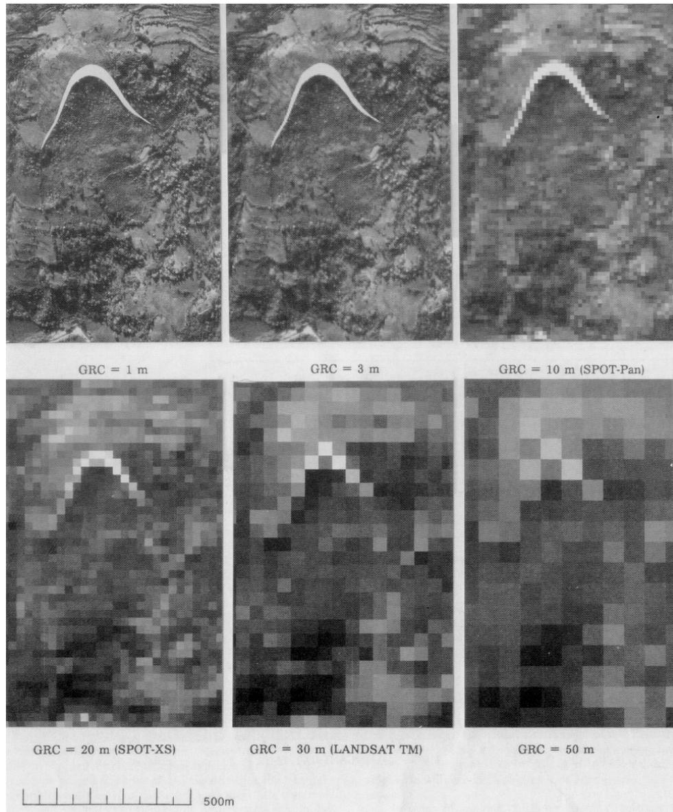
Figure 2: The same area as in the previous figure, but now with an artificially enhanced landslide scar.
