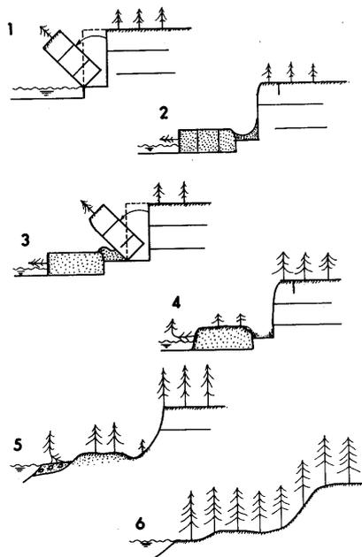
Figure 2.2: Landslide activity classes: 1: active, 2: suspended, 3: reactivated, 4: dormant, 5: stabilized, 6: relict.
