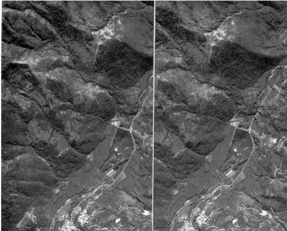
Figure 7: Major earth flow within small valley and almost blocking main valley. Convex form of earth-flow is characteristic of earth-flows and contrasts with concave forms of alluvial fans. River is pressed against opposite side of the valley and may cause undercutting and slope failures on that side.
