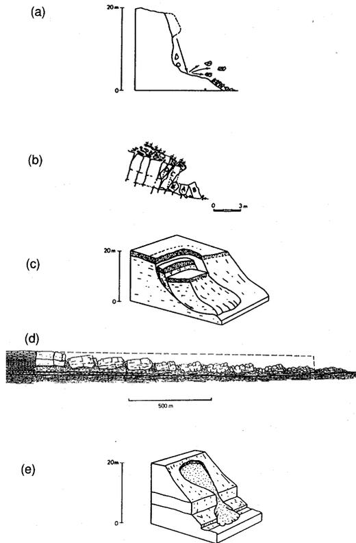
Figure 2.3: Landslide types: a: fall, b: topple, c: slide, d: spread, e: flow. (sagging is not indicated) (Varnes, 1978)
