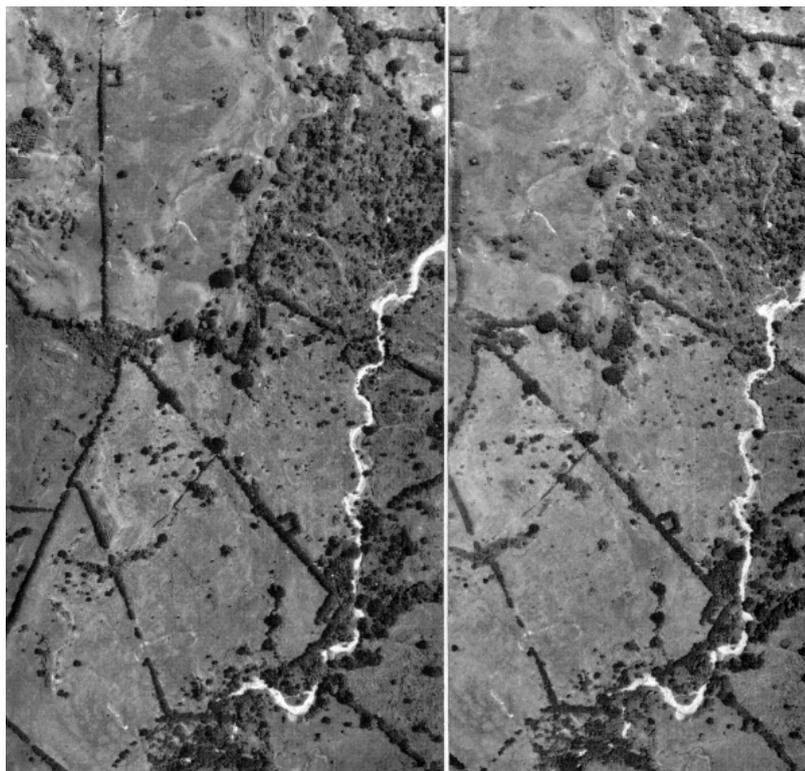
Figure ? : Highly unstable zone with numerous rotational landslides, mud slides, and earth flows. Well-cemented, but strongly jointed volcanoclastic sequence, dipping gently to the southwaet (north is up), overlies series of almost unconsolidated sandstones and mudstones and claystones, deposited in shallow marine to coastal environment. Steplike morphlogy is characteristic for rotational slides. Hummocky morphology is more indicative for flow-like movements.
