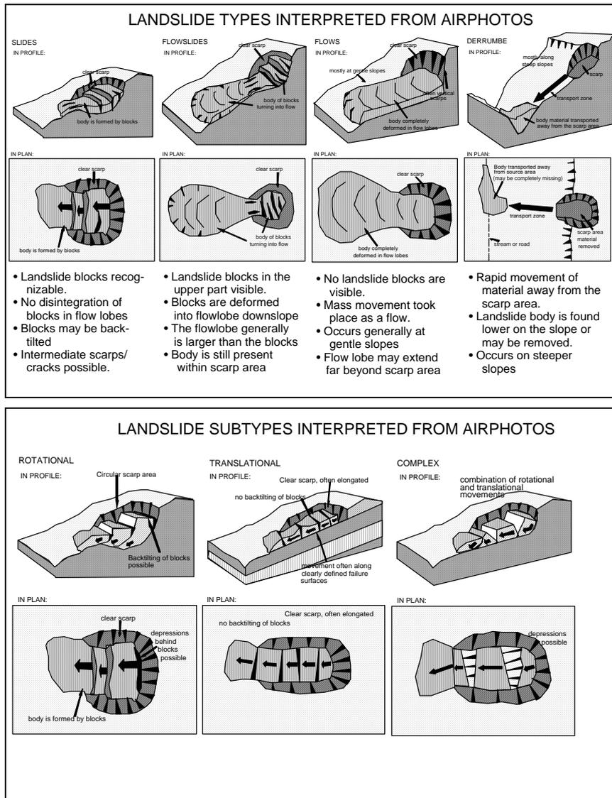
Figure 2: Some characteristics that can be interpreted from aerial photos that are used to describe landslide types and subtypes.
