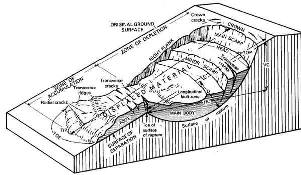
Figure 2.1: Block diagram of idealized complex earth slide-earth flow (Varnes, 1978)
