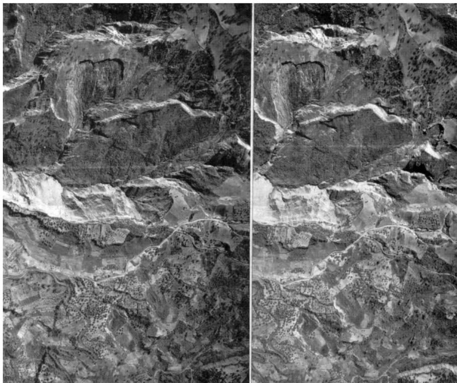
Figure ? : Translational slides controlled by dip slopes in sequence of very friable sandstones alternating with siltstones and mudstones. Joint controlled back scarp, linear patterns, and micromorphology of area where the sandstones have slid away (lower part) are diagnostic for landslides.
