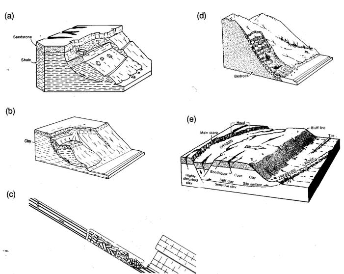
Figure 2.5: Different types of slides. a: rotational rock slide; b: rotational earth slide; c: translational rock slide (upper portion is rock block slide); d: debris slide; e: translational earth slide (Varnes, 1978)
