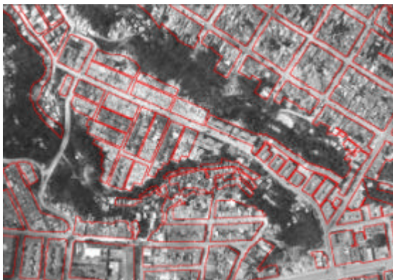
Figure 2. Digital orthophoto combined with existing cadastral data in the GIS
