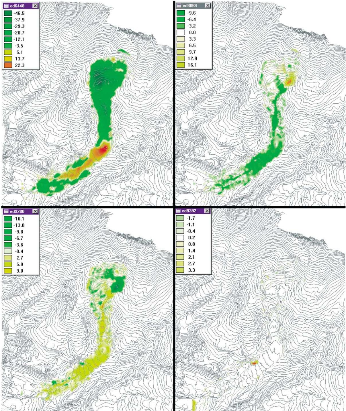
Fig. 6. Elevation difference between DEMs constructed from multitemporal contour maps. Upper left: 1964–1948. Upper right: 1980–1964. Lower left: 1992–1980. Lower right: 1993–1992.
