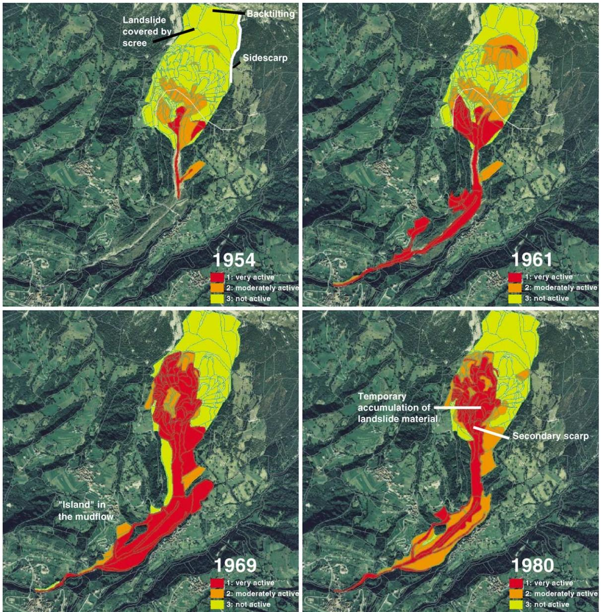
Fig. 4. Tessina landslide activity as mapped from aerial photographs. (A) Upper left, 1954. (B) Upper right, 1961. (C) Lower left, 1969. (D) Lower right, 1980.
