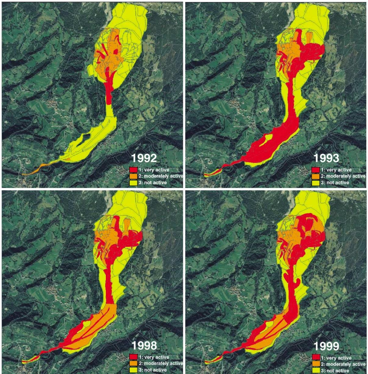
Fig. 5. Tessina landslide activity. (A) Upper left, in 1991/1992 as mapped from aerial photos. (B) Upper right, in 1993 as mapped from videomages and oblique photos. (C) Lower left, in 1998 as mapped in the field. (D) Lower right, in 1999 as mapped in the field.
