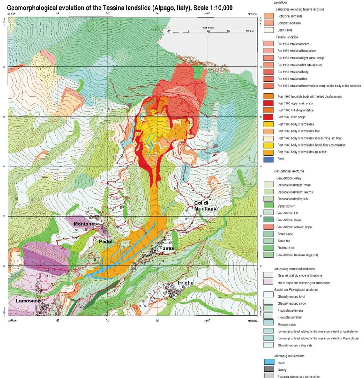
Fig. 3. Geomorphological map of the Tessina landslide area.
