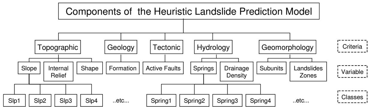
Figure 5: Components of the heuristic landslide hazard model.
