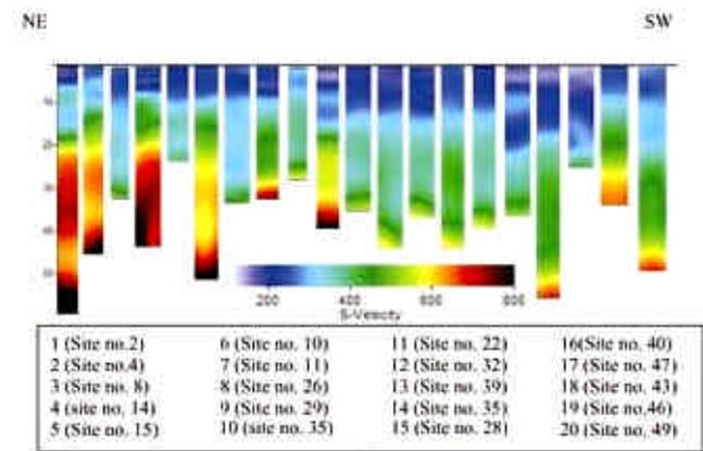
**Figure 8.** Shear wave velocity section for 20 sites located from northeastern to southwestern parts of the city indicating variation in depth of various soil layers. The top-most layer with a velocity of about 200 m/s is thin in northeastern part compared to the south-southwestern part of the city.
