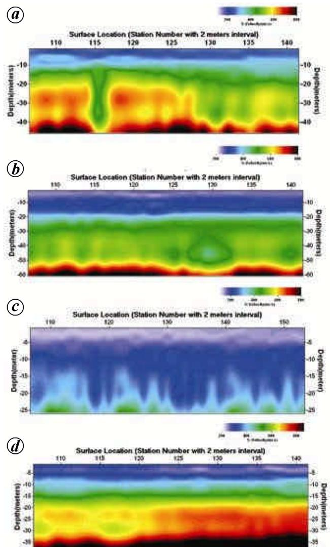
**Figure 6.** Shear wave velocity profile at (a) Anarwala (site no. 4) trending east-west, (b) Danda Nuriwala site (site no. 8) trending north-west-southeast, (c) Darawala site (site no. 40) trending south/southwest-north/northeast and (d) Badripur site (site no. 46) trending southwest-northeast.
