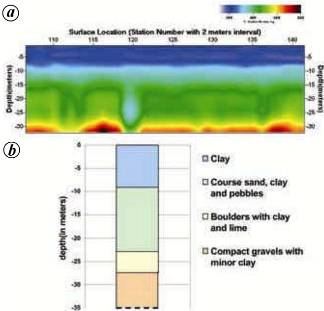
**Figure 7.** *a*, Shear wave velocity profile in the Forest Research Institute (FRI) site no. 26. The profile shows 10 m of upper layer having  $V_s$  of about 200 m/s that increases to 500 m/s at a depth of 30 m. The second layer is thick in this section compared to site no. 2. *b*, Tubewell litholog of a site close to FRI site no. 26 and corresponding  $V_s$  profile.
