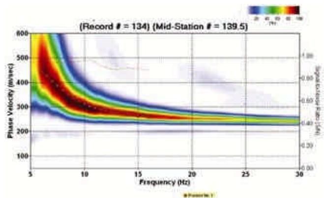
**Figure 4.** Dispersion curve (frequency vs phase velocity) depicting overtone image. For frequencies as low as 7 Hz, significant amount of energy of surface waves has been recorded using 14 Hz geophones from Danda Nuriwala site.
