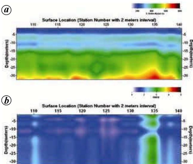
**Figure 5.** Shear wave velocity section at Surya Prasth Ashram (SPR) site no. 2) trending southwest-northeast.
