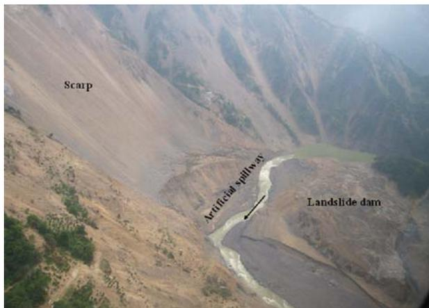
**Fig. 12** Helicopter view of the artificial spillway in the Tangjiashan landslide dam
