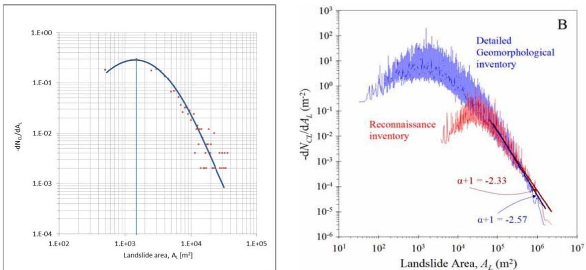
Figure 4-11: Left: Cumulative frequency-area distribution for landslide events in St Luci for the period 2010-2014 and Right: an example of the different cumulative frequency-area distributions for reconnaissance and for detailed geomorphological surveys (Guzzetti 2005).
