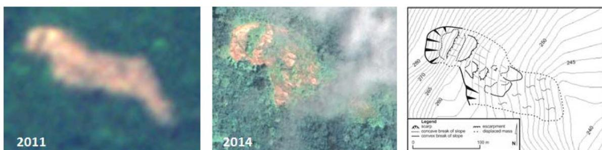
Figure 4-23: The 2011 image of a landslide enables establishment of just an outline of a landslide feature near the Roseau Dam. However, the 2014 Pleiades image can be used to draw a tentative morphological map of a landslide complex. Field checks are required to ensure these interpretations are realistic.
