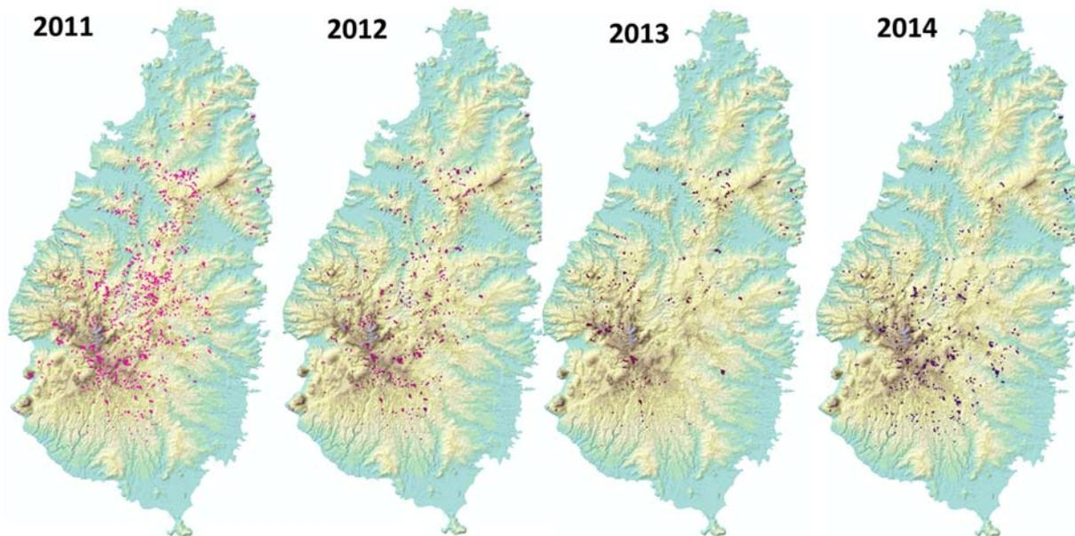
Figure 4-9: Landslide inventory maps of St Lucia showing the distribution of active landslides (NB identification is affected by cloud cover and a poor quality SE quadrant for 2013; see Table 3).
