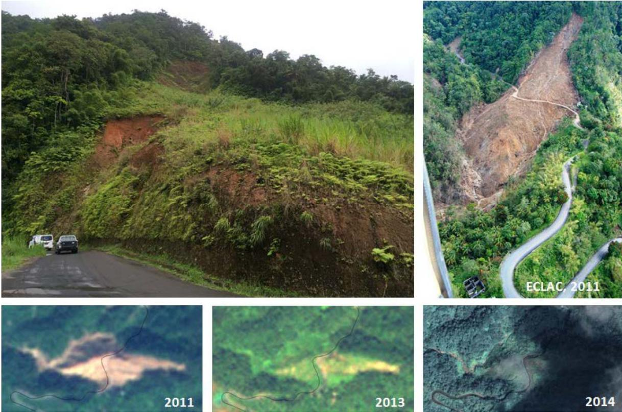
Figure 4-14: Colombette Landslide. Top left is the state of the upper part of the landslide in October 2014 and top right shows the landslide in 2011. The lower images represent scenes from RapidEye (2011 and 2013) and Pleiades (2014). Despite the greater resolution of the Pleiades image, the landslide is barely visible.
