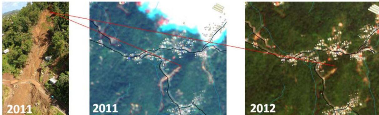
Figure 4-16: The landslide/debris flow event of Ti Rocher. To the left an oblique of the event is shown (source ECLAC 2011). The event is clearly visible on the 2011 RapidEye image, while only a year later all landslide deposits below the road are covered by vegetation.
