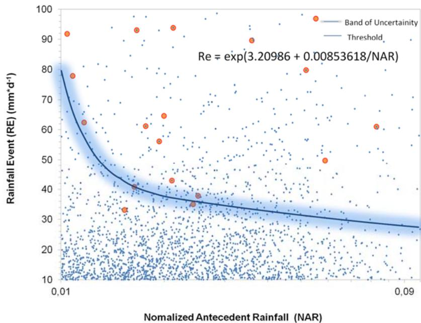
Figure 3-9: Landslide rainfall threshold for Dominica. RE is the threshold rainfall, and NAR is the 5-day antecedent rainfall; the orange points are the reported landslide events; blue points are the rainfall days without landslides, the blue line is the estimated rainfall threshold; the blurred blue area is the band of uncertainty which was visually identified.
