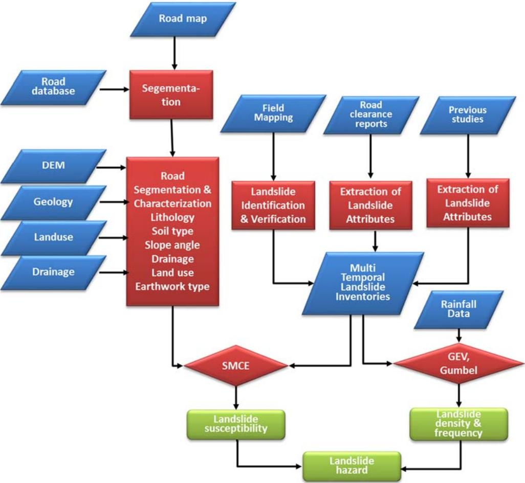
Figure 7-1: Method used for assessing the landslide susceptibility (and hazard) along the national road network in Saint Lucia. Landslide hazard is obtained by combining the susceptibility classification with the results of the density-frequency analysis.
