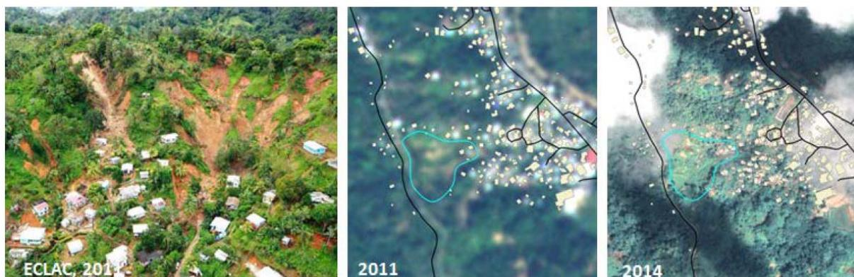
Figure 4-17: Landsliding near Marc. The oblique photo on the left (source ECLAC 2011) shows the extent of the area affected. The blue outlines in the 2011 image follow the outline of the valley. In the 2014 Pleiades image the landslide complex is barely recognisable.
