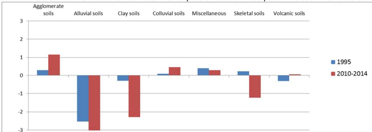
Figure 6-10: Contrast factors for soil units for landslides in 1995 and 2010\_2014
