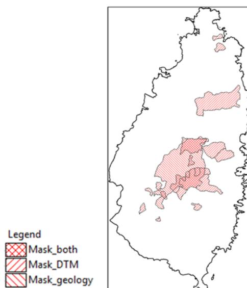
Figure 6-17: Areas where the quality of the landslide susceptibility map is less due to problems with the DEM, the geological map, or both.
