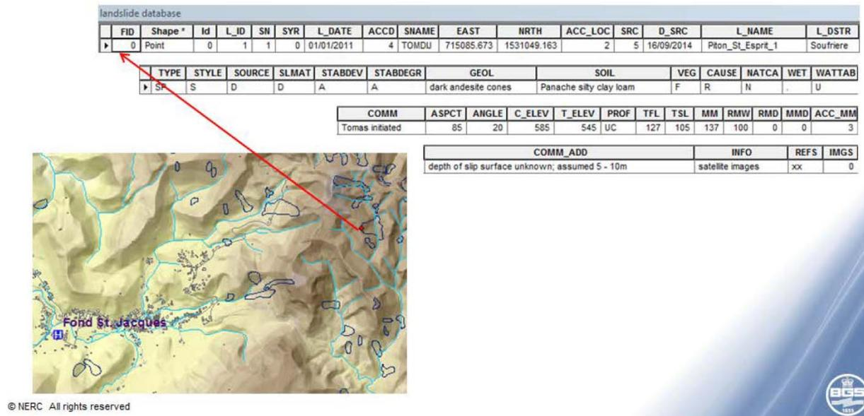
Figure 4-10: An example of additional point data that can be linked to each landslide polygon to build up a landslide database that can be used for further analysis (see Foster et al. 2012).
