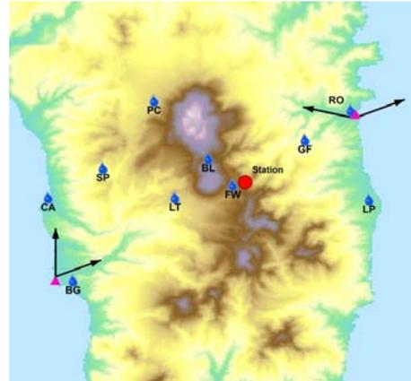
Figure 3-6: Location of 10 rain gauges installed for the DOMEX project at different altitudes and sides of the island in Dominica (Source: <http://www.domex2011.com/rain-gauge-network>)
