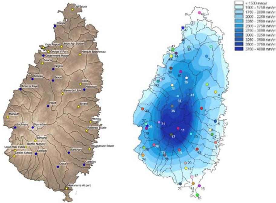
Figure 3-10: Rainfall stations on St Lucia. Left: stations represented as yellow dots are used in the frequency magnitude analysis (1955-2005). Right: average annual rainfall, ranging from 1500 mm/year (white) to 4000 mm/y (dark blue), by Marmagne and Fabrègue (2013)
