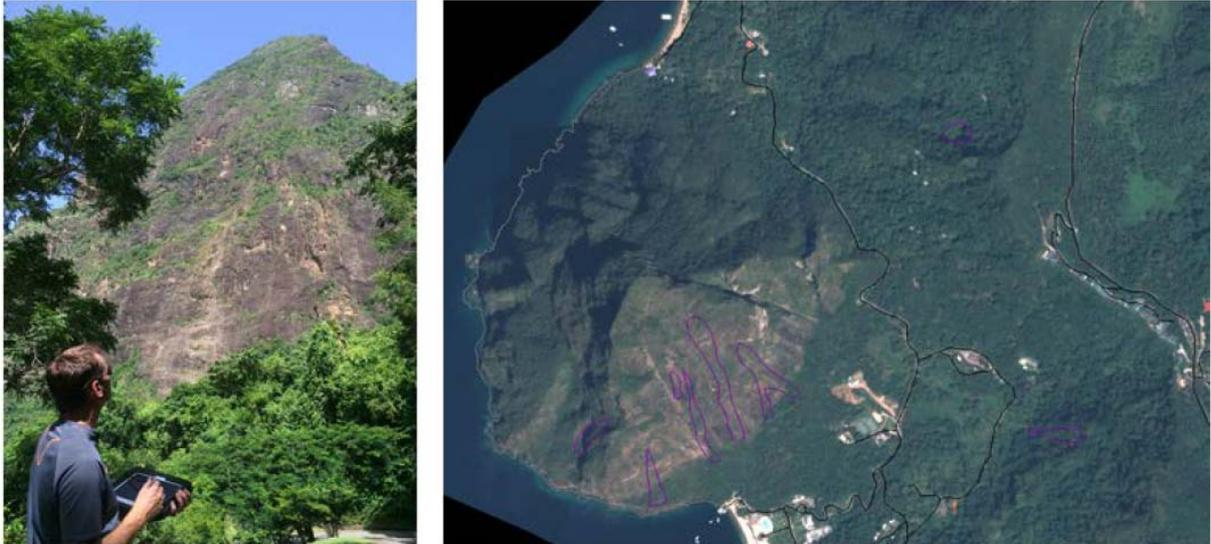
*Figure 4-18: The Petit Piton with fresh trails of rockfalls and the 2011 rockfall trails superimposed on the 2014 Pleiades image. In the SE corner of the image landslide trails were observed in the field (Figure 4-19) but these could not be identified on the satellite images.*
