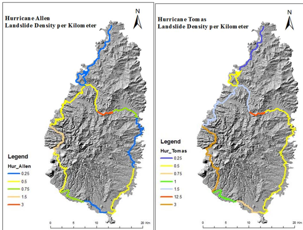
Figure 7-3. The results of the study by Mott MacDonald (2013) on landslide density per kilometer road. Post hurricane Allen (left) and post hurricane Tomas (right).
