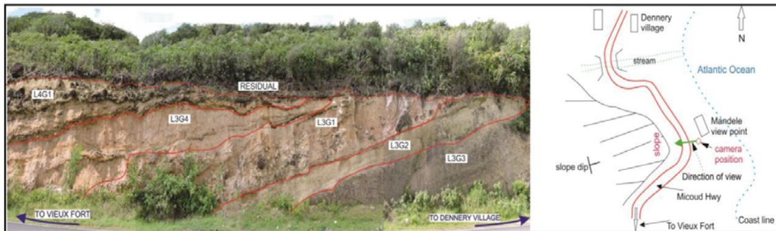
Figure 5-4. Example of an outcrop in volcanic deposits, and the separation into different geotechnical Units (Mulenga, 2015).
