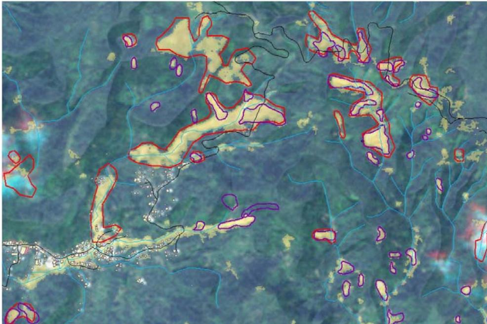
Figure 4-13: The Fond St Jacques/Migny area on the 2011 RapidEye image. The light coloured pixels indicate the result of a 'bare earth' classification (areas larger than 300 m<sup>2</sup>). The red polygons represent the 2010 landslide inventory and the purple polygons the multi-temporal inventory where bare earth signatures in valleys and fields have not been included. The two landslide polygons in the centre were generated in 2014.
