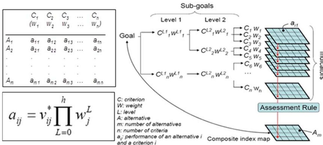
Figure 6-13: Schematic procedure for spatial multi-criteria evaluation based on the analytical hierarchical process
