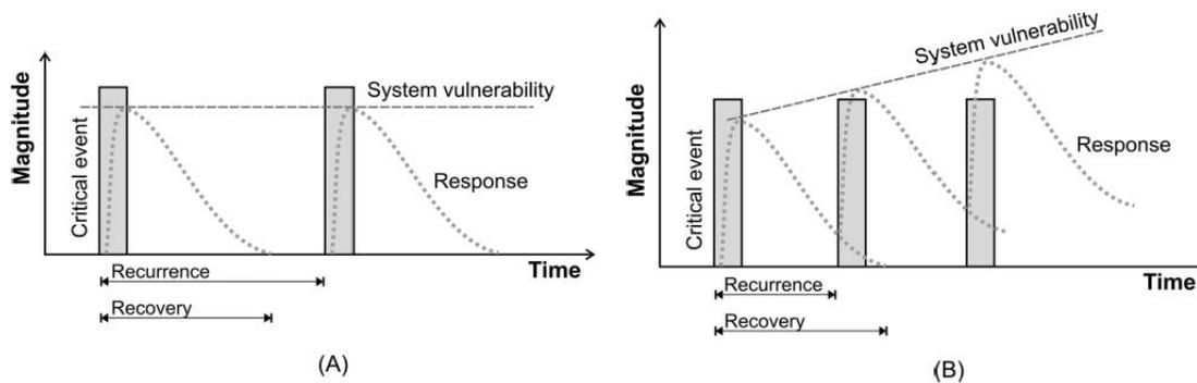
Figure 4-7. Landscape recovery versus trigger event recurrence. When recurrence exceeds recovery, relatively stable system vulnerability can be assumed (A), but when recovery exceeds recurrence, system vulnerability is likely to increase significantly. (From Dijkstra et al., 2014)
