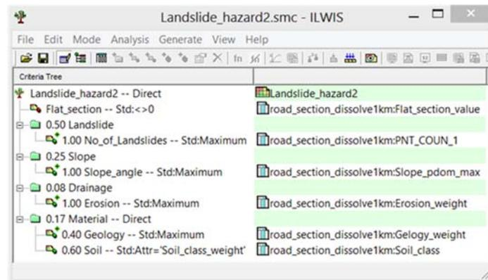
Figure 7-4: Criteria tree for analysing landslide susceptibility along the road network in Saint Lucia
