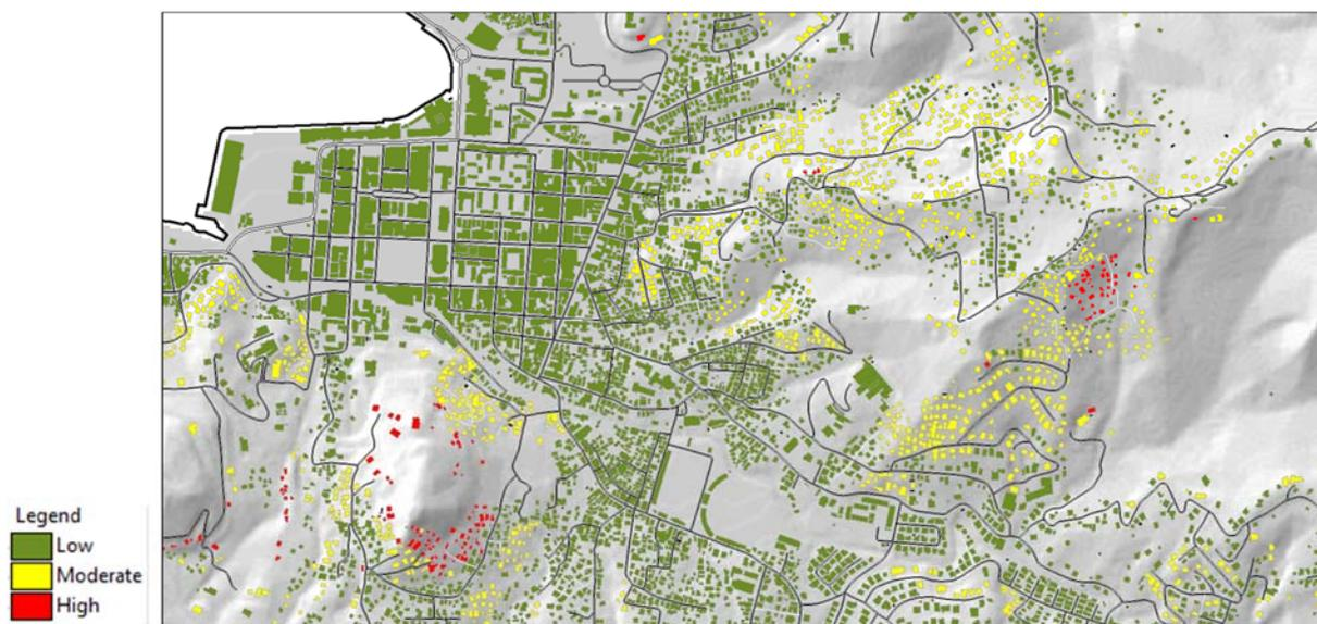
Figure 8.1: Landslide susceptibility of buildings in the area of Castries, based on the national scale landslide susceptibility map. Note: this map is not suitable for analysing local and site investigation scale
