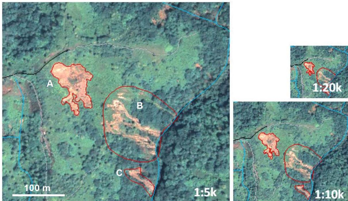
*Figure 4-20: An example of mapping at different scales at Chateau Belair using the 2014 Pleiades satellite image as an example (see also Figure xx for an indication of image variability across the multi-temporal image stack). At 1:5,000 scale it is possible to create a detailed outline of freshly exposed soils of a landslide (A), at 1:10k it is possible to roughly outline a small event (C) while at 1:20,000 scale a small cluster of linked events is grouped together (B).*
