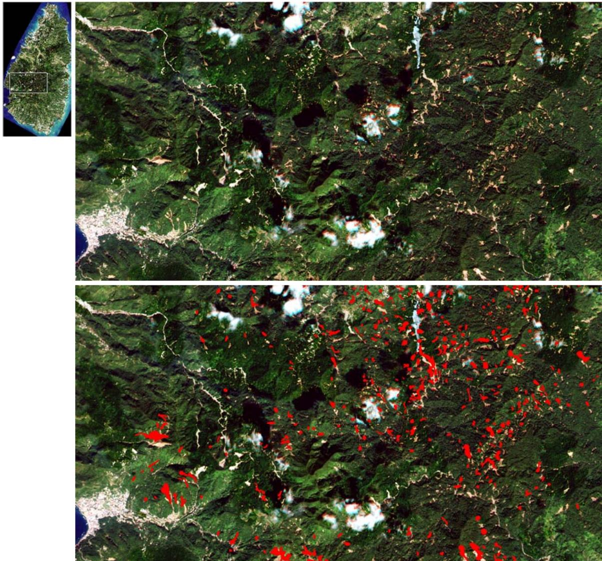
Figure 4-2: RapidEye image from 2011 showing the large number of landslides triggered by the 2010 Hurricane Tomas, and which was used by Abrahams and Rock to map the landslides. Note the distortion in landslide location due to problems in georeferencing the satellite image.
