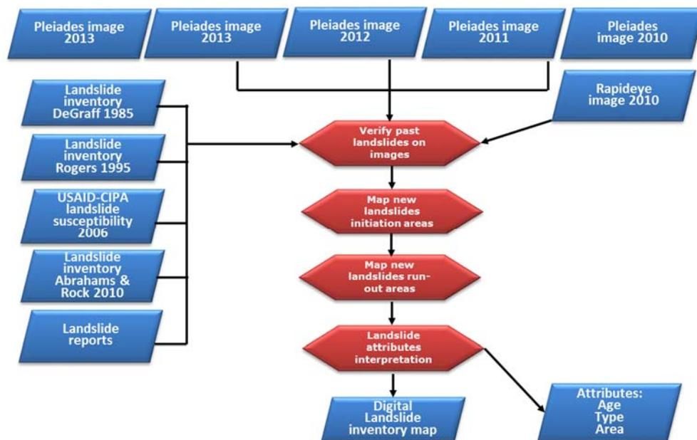
Figure 4-5: Schematic representation of the procedure followed from landslide inventory mapping in Saint Lucia by BGS (Jordan et al., 2015).
