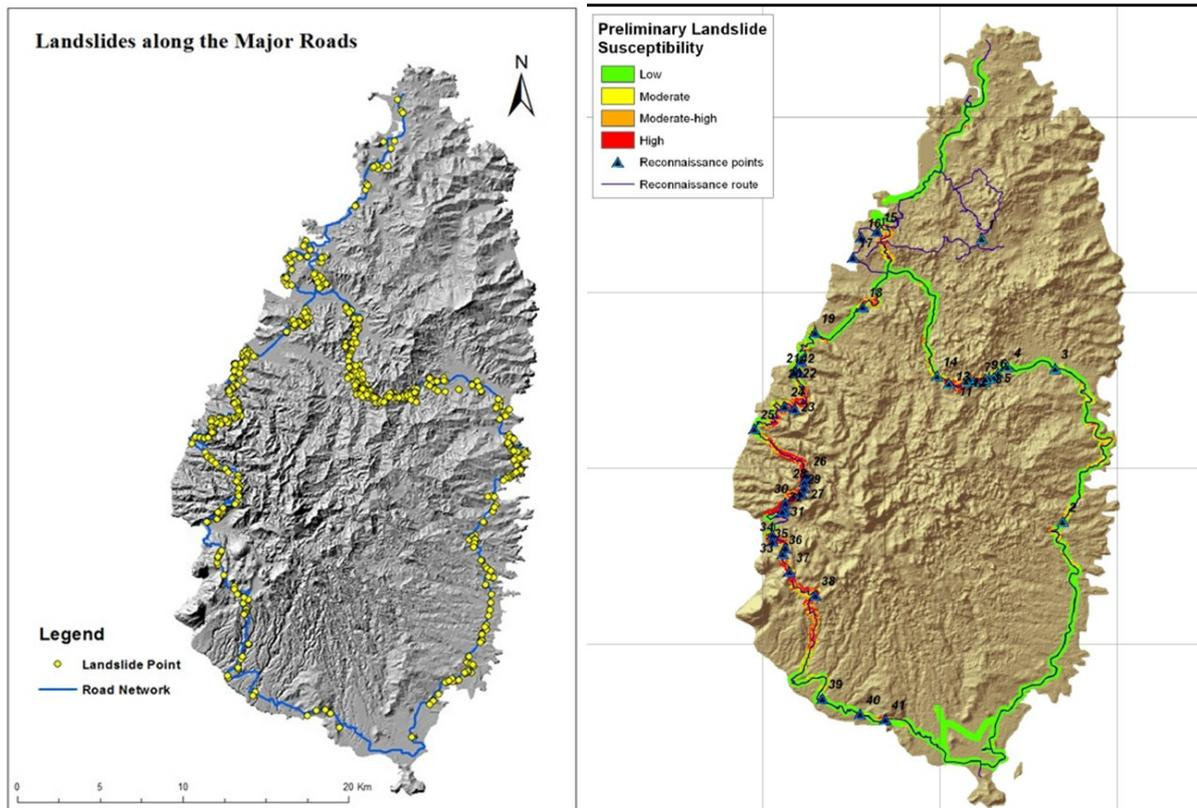
Figure 7-2: Left: Landslides along the Major roads of Saint Lucia. Source: Mott MacDonald (2013). Right: Preliminary landslide susceptibility map of the road network prepared by BGC (2012)
