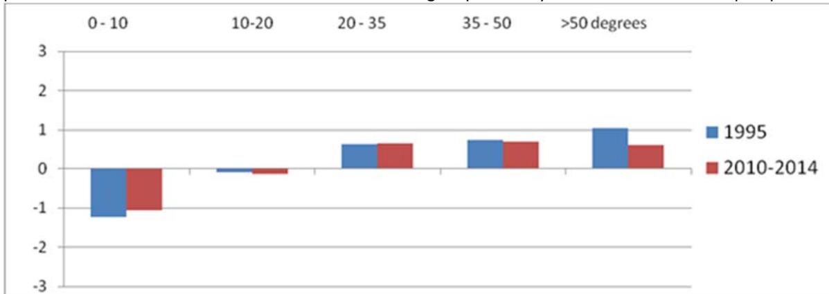
Figure 6-4: Contrast factors for slope steepness classes for landslides in 1995 and landslides in 2010\_2014
